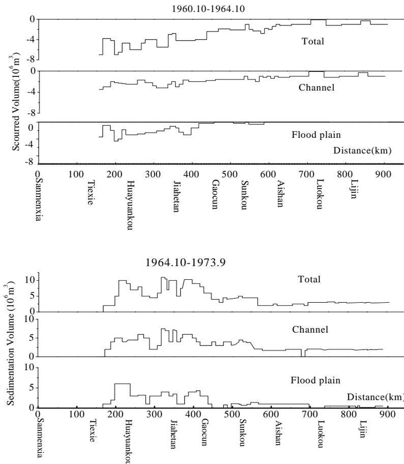
**Fig. 8** Volume of Sediment Erosion (from 1960 to 1964) and Resiltation (from 1964 to 1973) per Length in the Lower Reaches Downstream of the Sanmenxia dam. The Erosion and Resiltation Occurred Mainly in the Reach About 180km-600 km Downstream of the Dam (Yang *et al.*, 1994)
