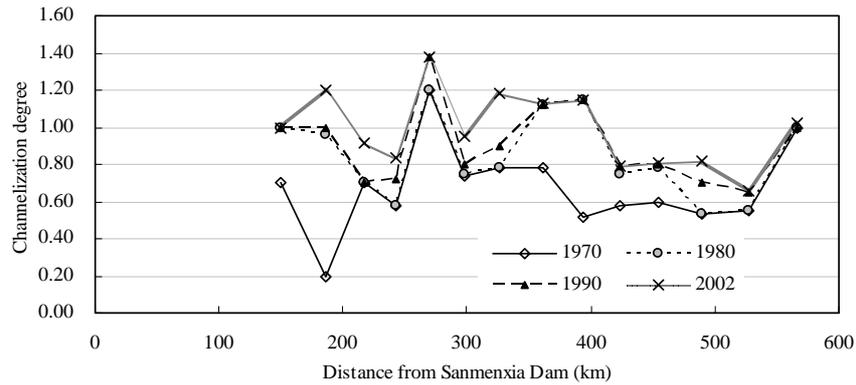
**Fig. 12** Distribution of Channelization Degree Along the Lower Yellow River (= Ratio of the Length of the Spur Dykes to the Length of the Channel)
