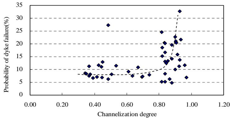
**Fig. 13** Probability of Dyke Collapse as a Function of the Channelization Degree
