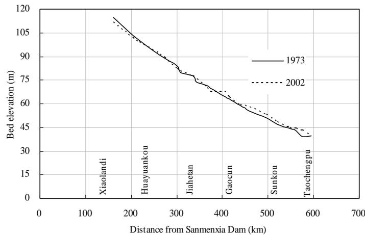
**Fig. 17** Longitudinal bed Profiles of The Lower Yellow River in 1973 and 2002
