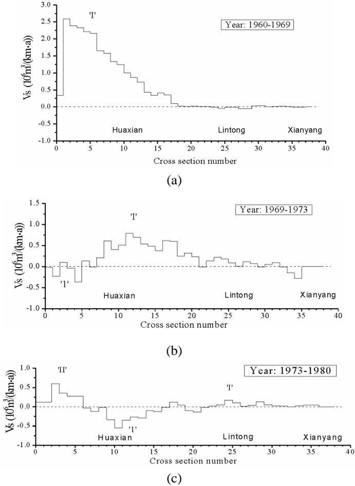
**Fig. 5** Erosion (-) and sedimentation (+) per unit length per year showing retrogressive waves in the lower Weihe River, as a result of ascent and descent of the Tongguan elevation. (The cross sections are numbered from the river mouth. Huaxian, Lintong and Xianyang are cities by the river. The distance between neighboring cross sections is about 6 km.)
