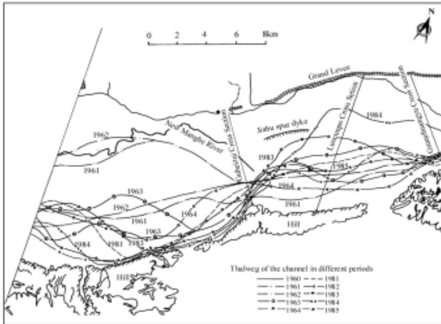
**Fig. 9** The Lower Yellow River Channel Wandered within the Grand Levees During the Storage Operation (1960-1964) and Late Operation Periods (1980-1984) of Sanmenxia Dam. (The Curves are the Thalweg of the Channel in Different Periods.)
