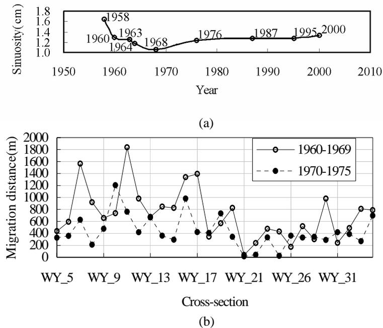
**Fig. 6** (a) Variation of sinuosity of the lower Weihe River (The closure of Sanmenxia dam in 1960 caused an abrupt reduction in the sinuosity). (b) Migration distances of the stream channel measured at cross-sections WY5-WY35 during the first ascending and first descending periods of Tongguan’s Elevation.
