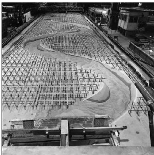
Fig. 13. Main channel bedforms—roughened floodplains—for flow of  $0.600 \text{ m}^3/\text{s}$
