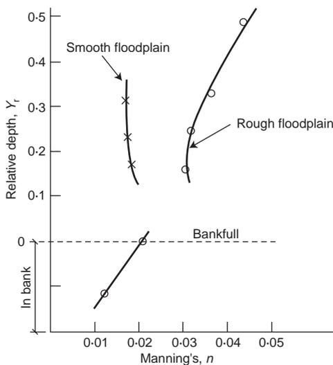
Fig. 8. Variation of single-channel Manning's  $n$  with depth
