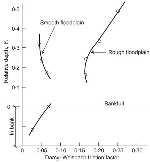
Fig. 9. Variation of single-channel friction factor with depth
