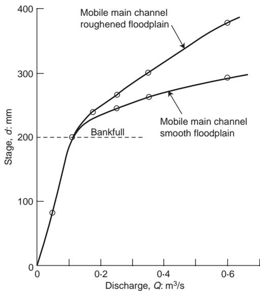
Fig. 3. Stage-discharge curves—inbank and overbank flow
