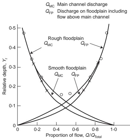
Fig. 7. Proportions of flow in main channel and floodplain
