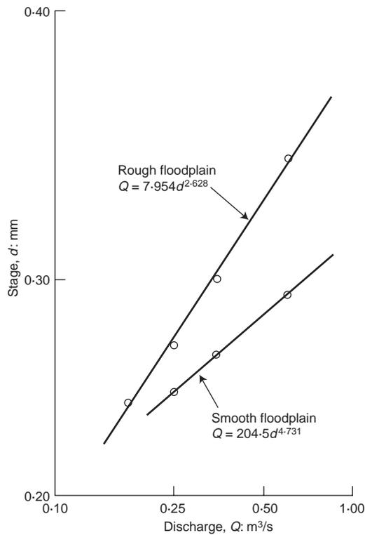
Fig. 4. Stage-discharge relationships—overbank flow
