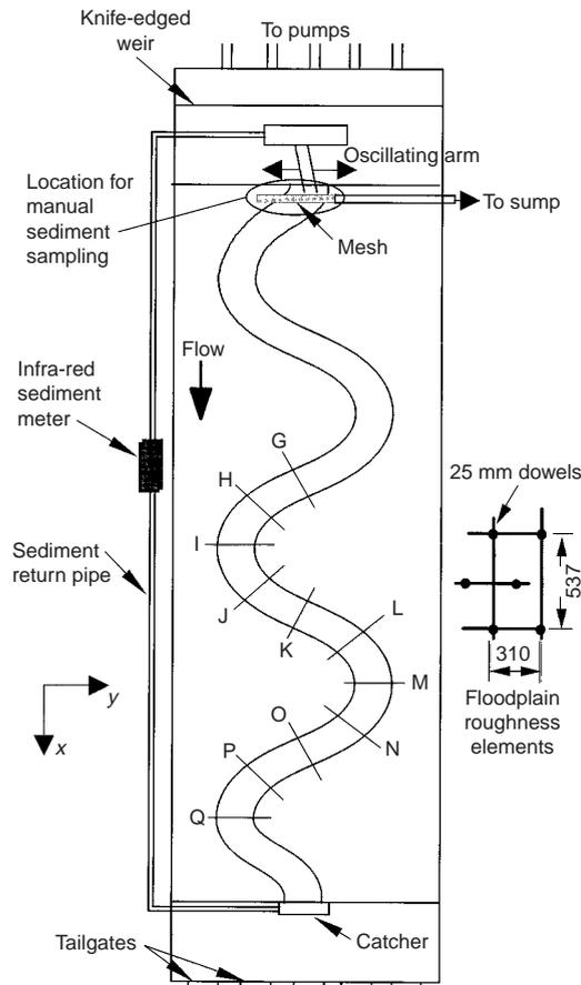
Fig. 1. Experimental arrangement at the FCF
