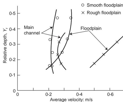
Fig. 6. Average velocities in main channel and floodplain
