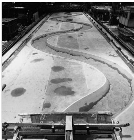
Fig. 12. Main channel bedforms—smooth floodplains—for flow of  $0.600 \text{ m}^3/\text{s}$
