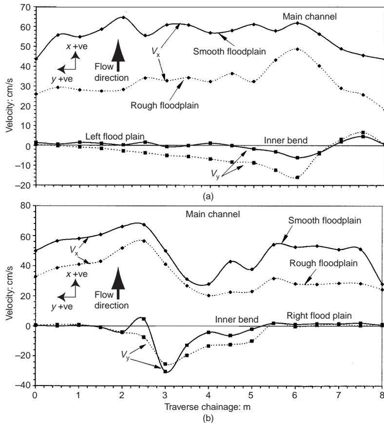
Fig. 5. Floodplain depth-average velocity components for: (a) apex I; and (b) cross-over O (discharge =  $0.350 \text{ m}^3/\text{s}$ )
