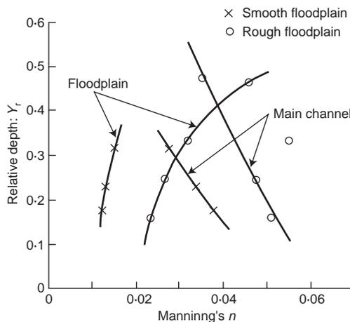
Fig. 10. Manning's  $n$  for main channel and floodplain
