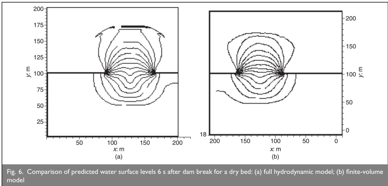
The solution is based on a second-order total variation diminishing (TVD) scheme and the model deploys an unstructured triangular grid.
