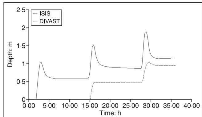
Fig. 14. Comparison of simulated flood depth time series at a point on floodplain
