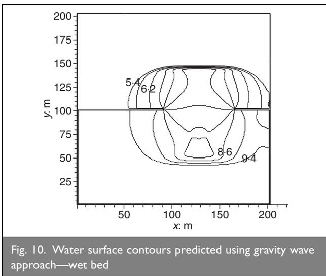
Fig. 10. Water surface contours predicted using gravity wave approach—wet bed
