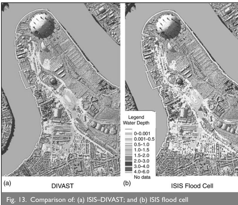
Fig. 13. Comparison of: (a) ISIS-DIVAST; and (b) ISIS flood cell
