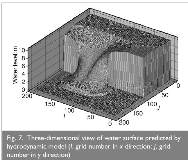
zero. There is a significant discrepancy between the predictions made by the model both with and without the advective term, see also Fig. 6. When the advective terms were neglected, then the propagation speed of the wave front was reduced. Using the flood wave approach, the predicted wave speed was significantly smaller than that using the gravity approach.
