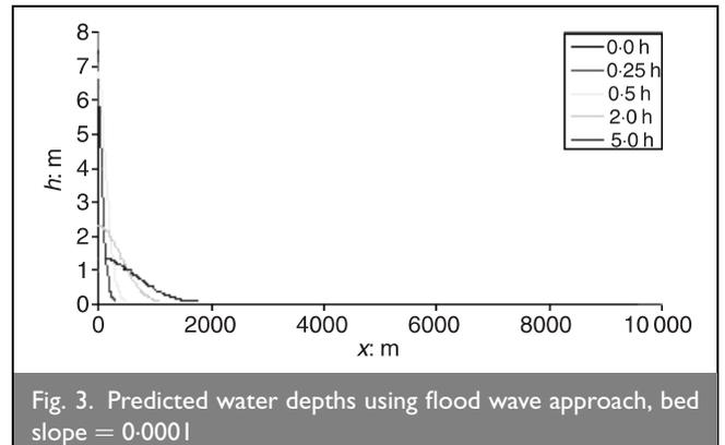
The length of the channel was set to 10 000 m, and the width was assumed to be 100 m. Two channel bed slopes were tested, namely  $S = 0.001$  and  $S = 0.0001$ , and the channel was initially assumed to be dry for both of these two cases. A sinusoidal hydrograph was used to represent the flood wave after the breaching of a dam, giving<sup>7</sup>
