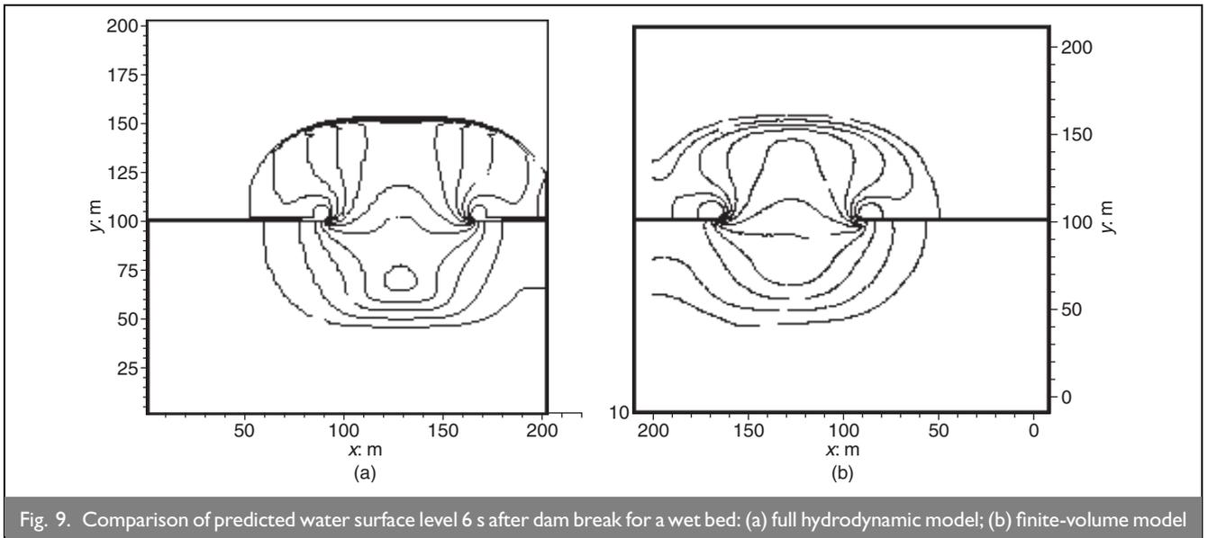
Fig. 9. Comparison of predicted water surface level 6 s after dam break for a wet bed: (a) full hydrodynamic model; (b) finite-volume model
