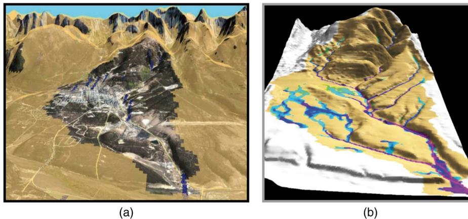
Fig. 2. Flow depth from *TRES* at California Gulch, Colorado, during 100-year storm
