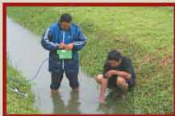
Velocity Measurement in Swale
