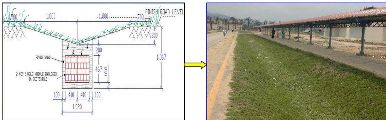
**Figure 5.0 : Ecological swale cross section and the completed ecological swale**
