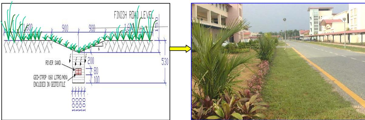
**Figure 4.0 : Perimeter swale cross section and the completed perimeter swale blended with the landscaping**
