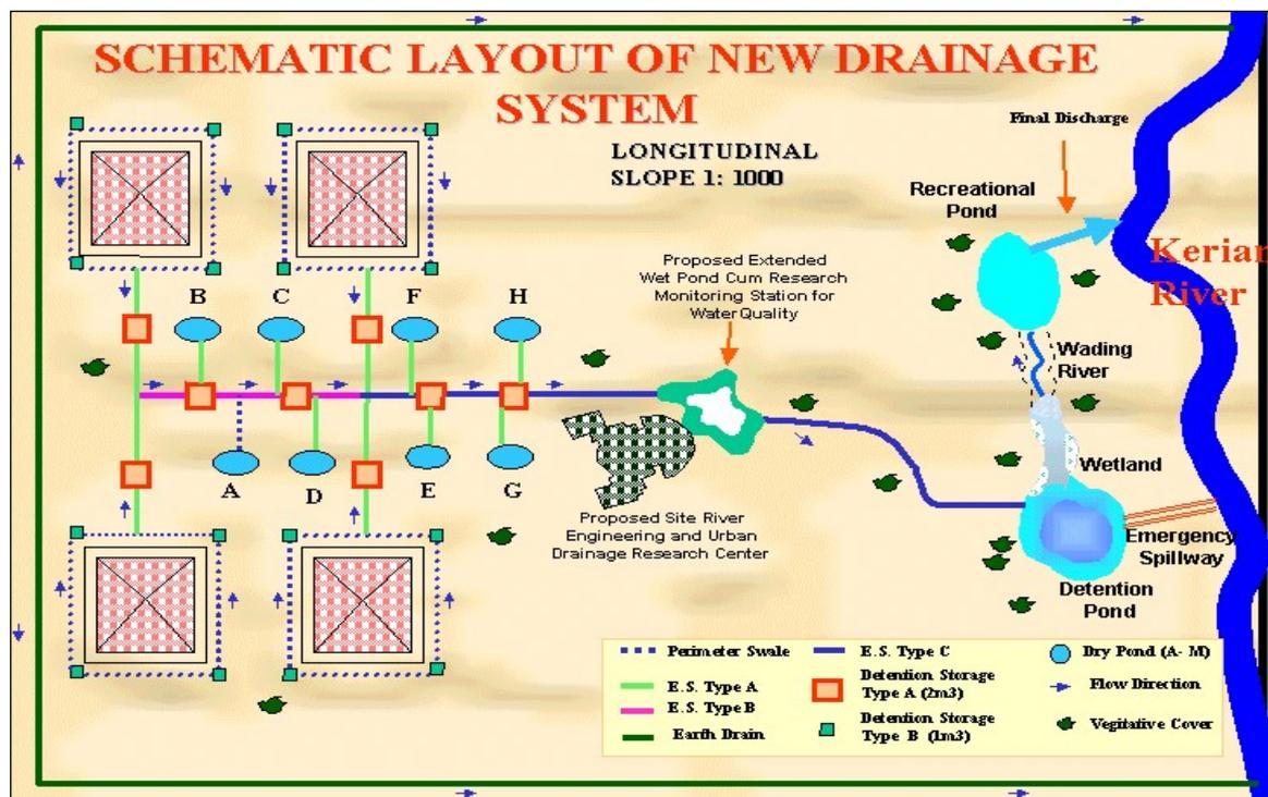
Figure 3. Schematic layout of Bio-ecological drainage systems (BIOECODS)
