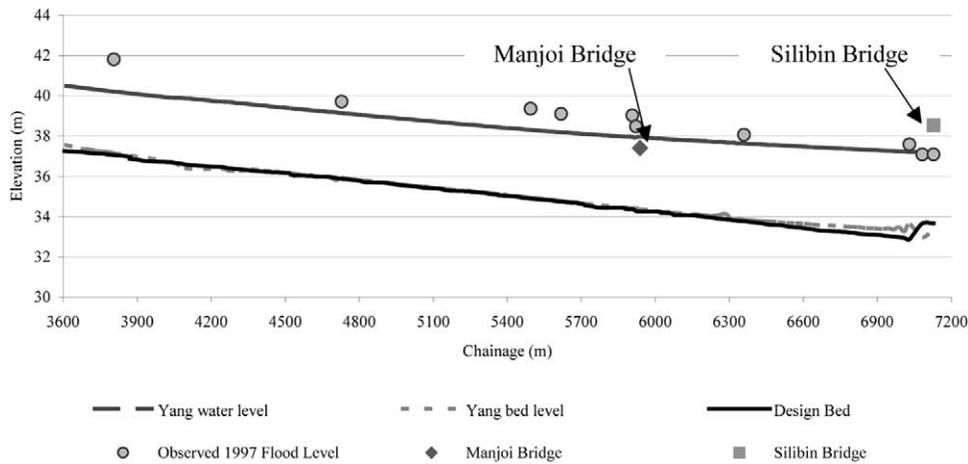
Fig. 8. The results of the calibration of HEC-6 using Yang equation (Tan, 2000).
