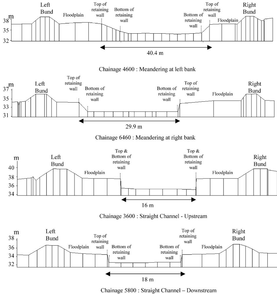
Fig. 5. Typical cross-section for Pari River.
