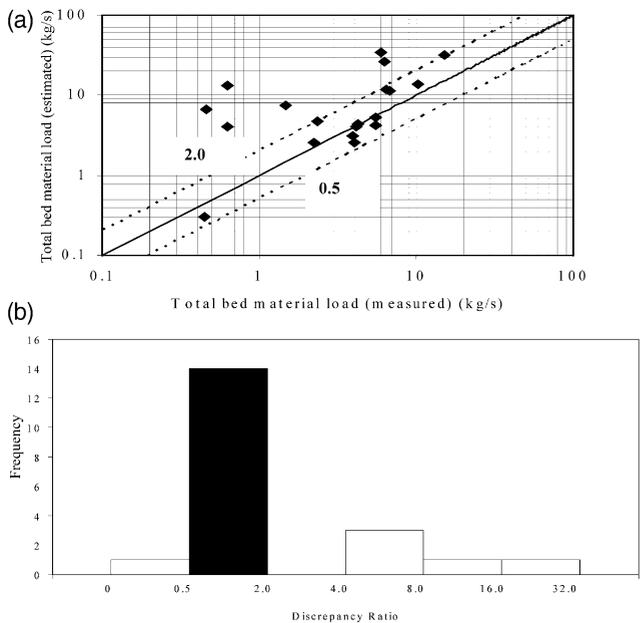
Fig. 9. Discrepancy ratio for sediment discharge at Pari River using Yang Equation (Yahaya, 1999).
