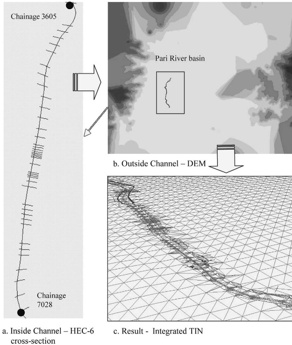
Fig. 12. Three-dimensional TIN terrain modeling approach.
