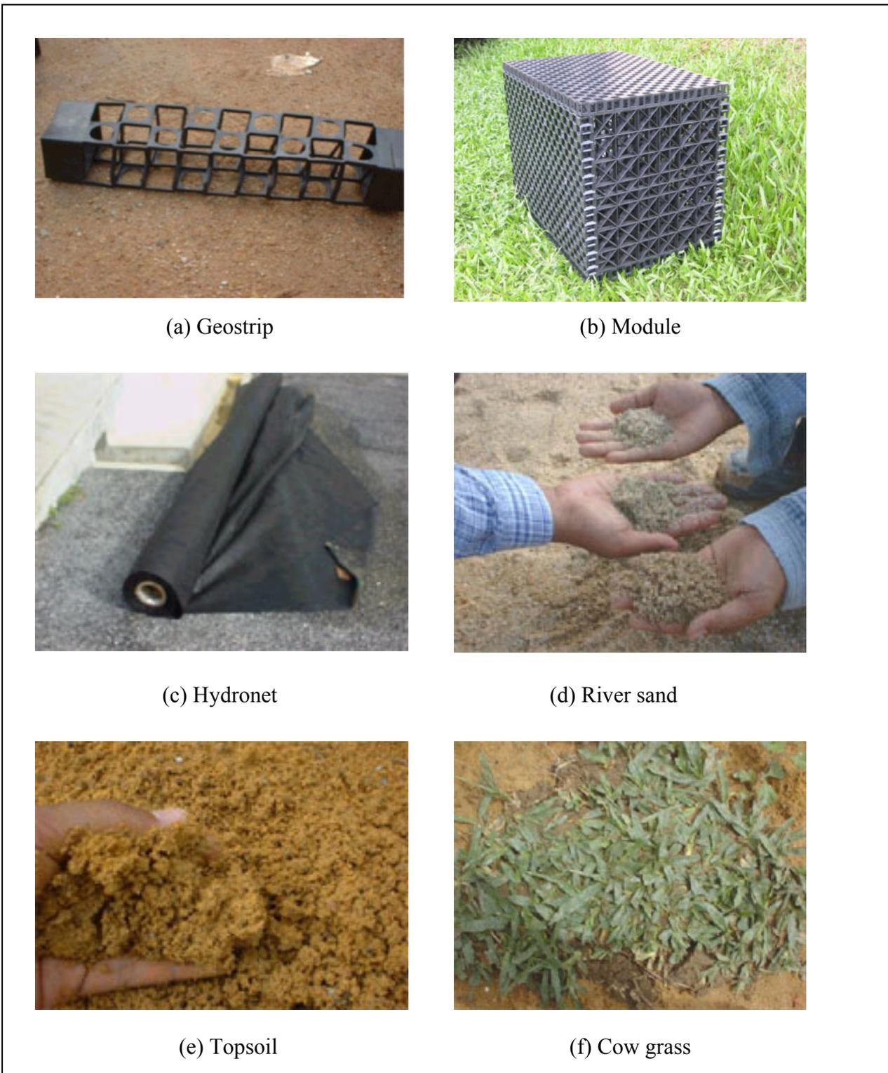
Figure 10 Components of an ecological swale
