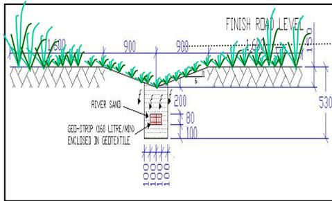
Figure 3a Typical cross section of perimeter swale
