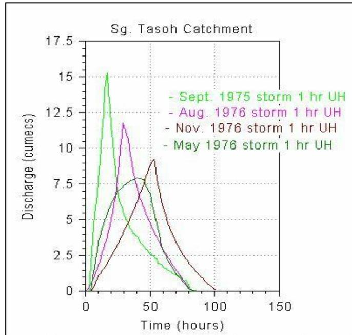
Figure 3 Curvilinear 1 hour Unit Hydrograph for Storms in Sungai Tasoh Catchment.
