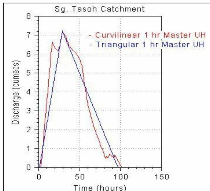
Figure 4 Curvilinear and triangular 1 hour Master Unit Hydrographs for Sungai Tasoh Catchment.
