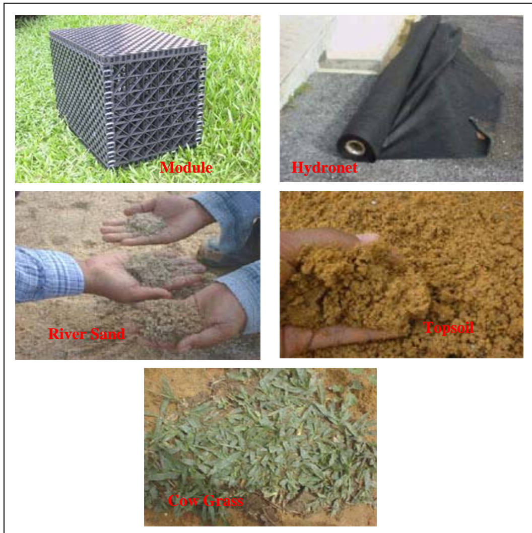
Figure 6 The material of construction of BIOECODS.
