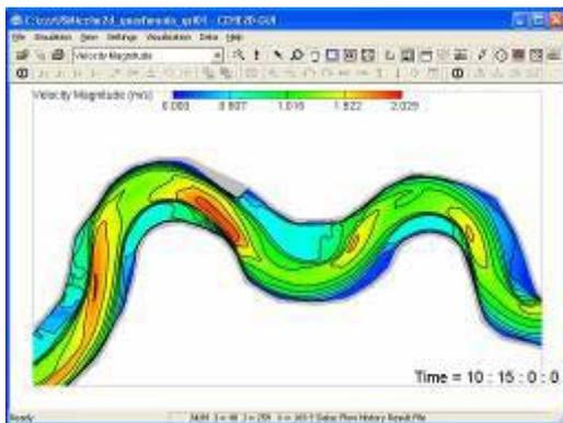
Figure 9 Velocity Contour
