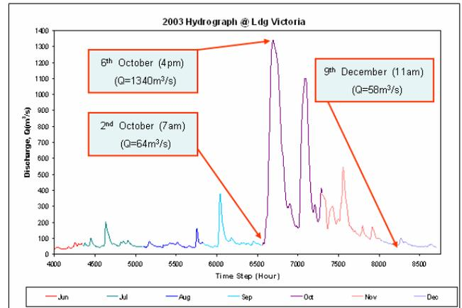
Figure 5 Input Hydrograph @ Ladang Victoria for Flood 2003
