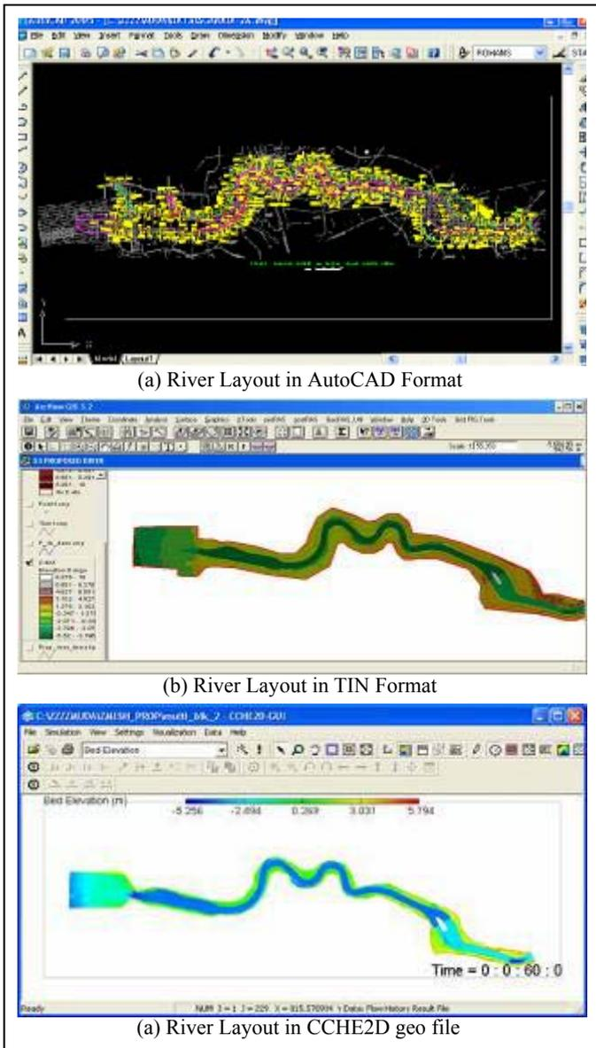
Figure 4 Processing AutoCAD to CCHE2D geo file
