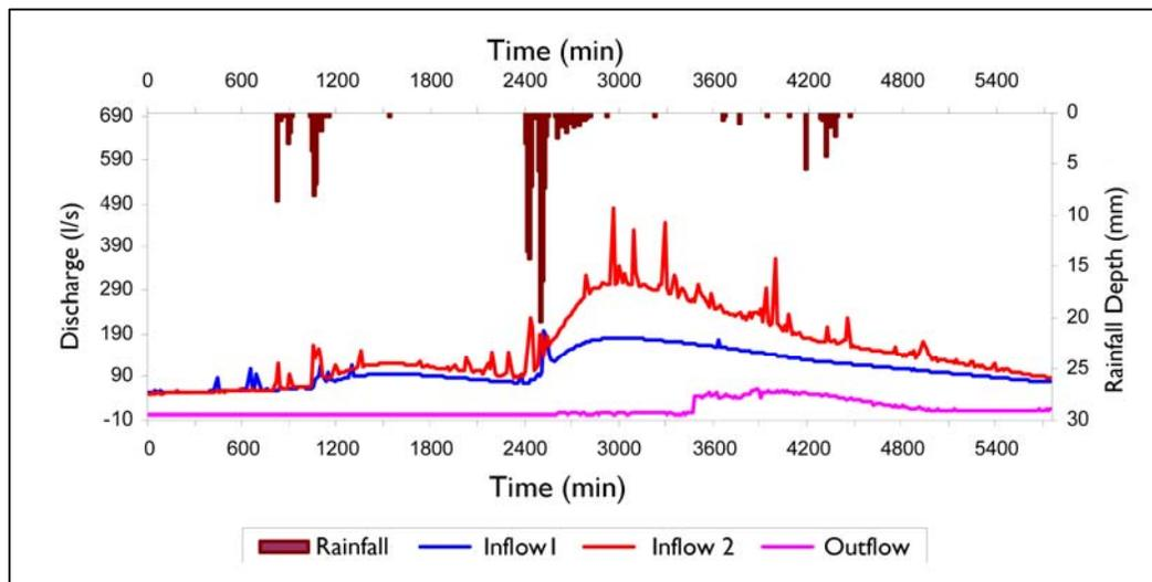
**Figure 4.** Peak flow attenuation during a 100-year event (21<sup>st</sup> - 24<sup>th</sup> July 2007).
