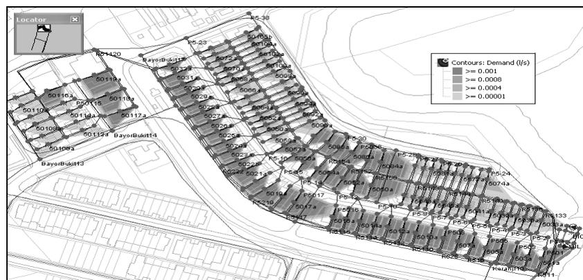
Figure 8: Network with Ecological Sanitation at Peak 1200 Hour of Average Working Day
