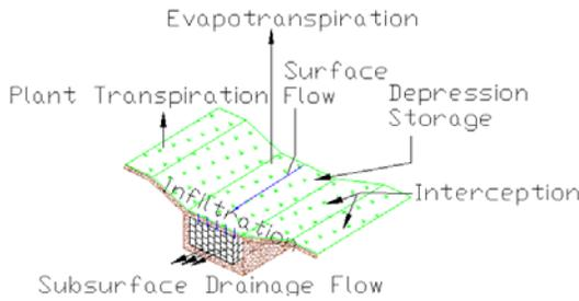
Figure 3. Processes occur in an ecological swale system.
