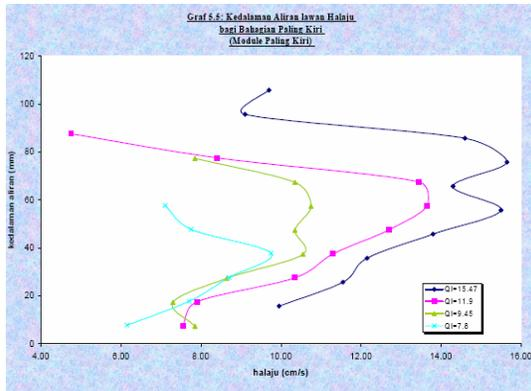
Figure 6. Relationship between flow depth and velocity in the drainage module (Mohd Sidek et al. 2002).
