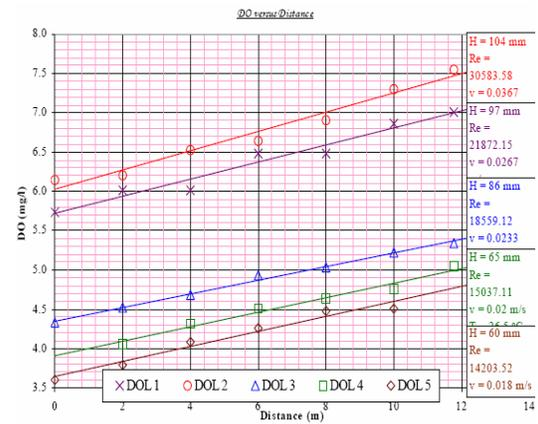
Figure 8. Relationship between dissolved oxygen and distance in the drainage module (Mohd Sidek et al. 2002).
