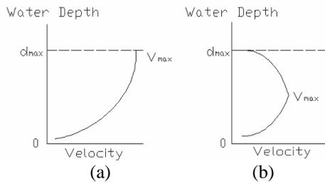
Figure 7. Relationship between water depth and velocity for: (a) open channel and (b) pipe.
