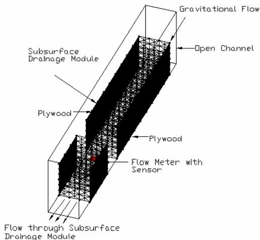
Figure 11. Laboratory test for subsurface module.
