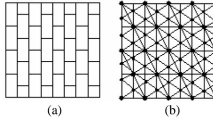
Figure 12. Side view of drainage module pattern for: (a) pre-existing subsurface drainage module (size 405 x 465 x 607) and (b) latest subsurface drainage module (size 410 x 450 x 685).
