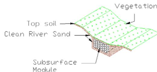
Figure 2. Isometric of ecological swale.
