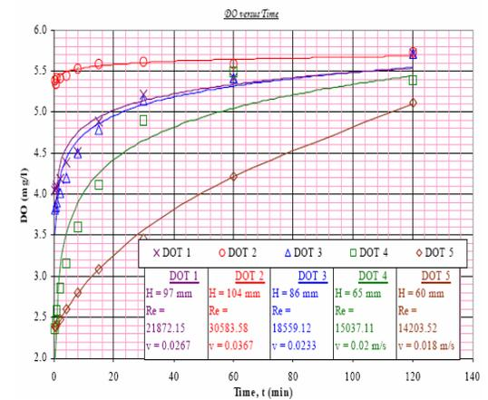
Figure 9. Relationship between dissolved oxygen and time in the drainage module (Mohd Sidek et al. 2002).
