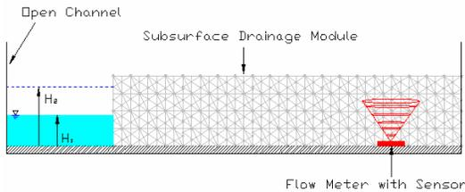
Figure 10. Conceptual view of the automatic velocity measurement system for flow in subsurface drainage module.
