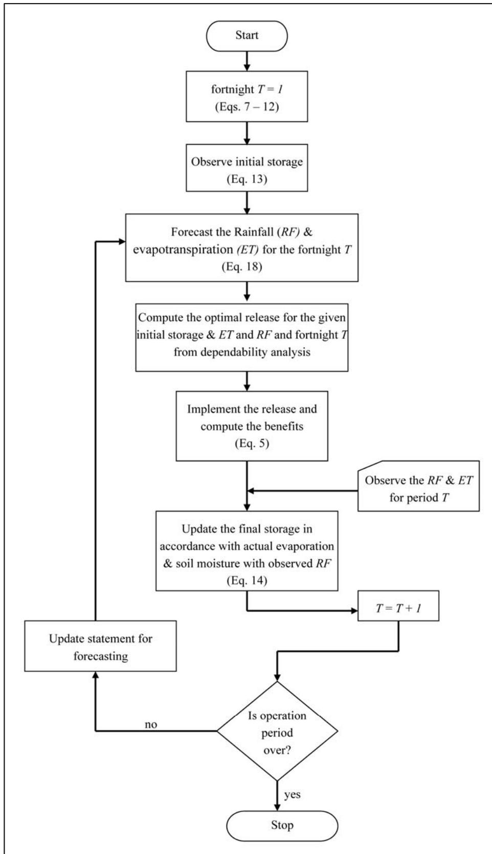
Figure 3 Flow chart of real-time operation of reservoir
