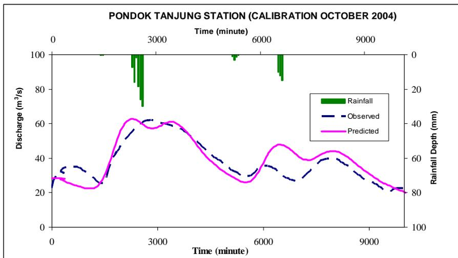
Figure 4 Runoff hydrograph for R40 at Pondok Tanjung discharge station (Calibration)
