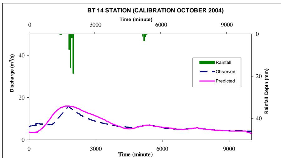
Figure 5 Runoff hydrograph for JR130 at Batu 14 discharge station (Calibration)
