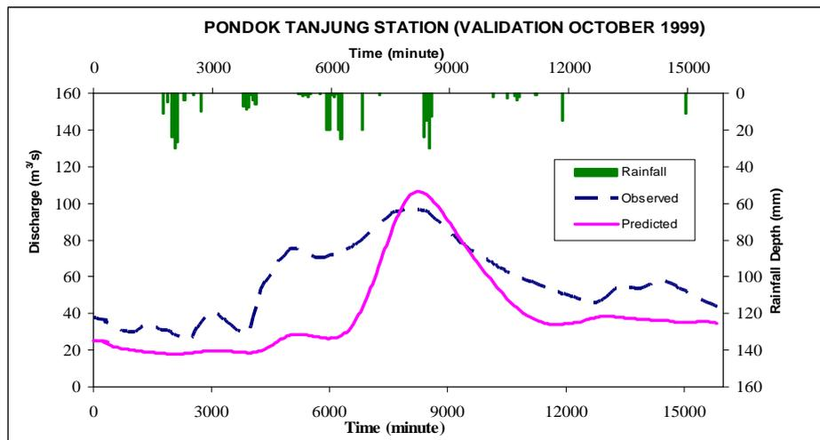
Figure 6 Runoff hydrograph for R40 at Pondok Tanjung discharge station (Validation)
