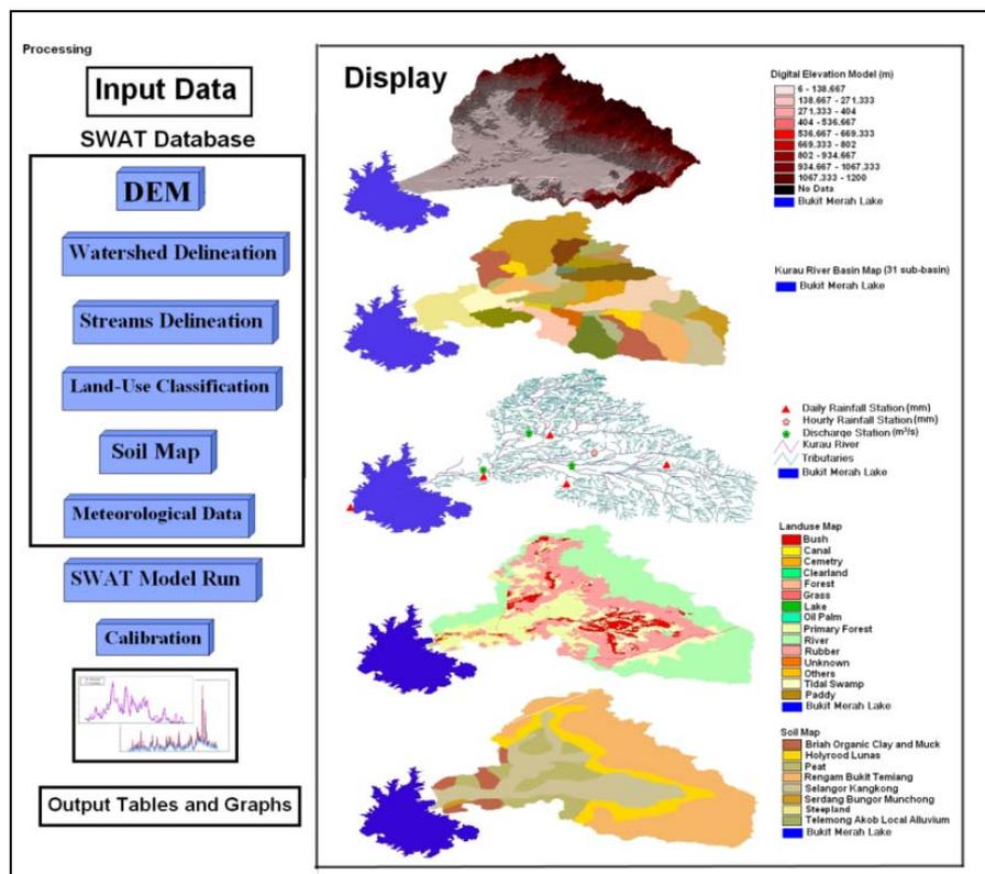
Figure 3 Schematic of SWAT processing for Kurau River
