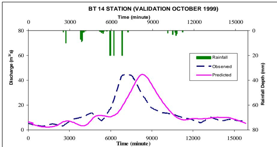
Figure 7 Runoff Hydrograph for JR130 at Batu 14 discharge station (Validation)
