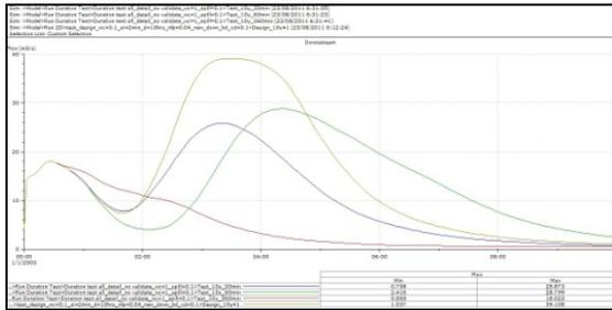
Figure 11 Discharge at downstream for different rainfall duration
