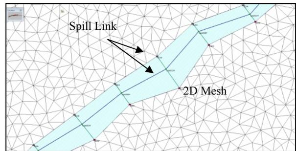
Figure 14 2D Mesh and Spill
