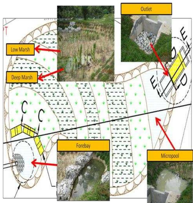
Figure 5: Component of constructed wetland
