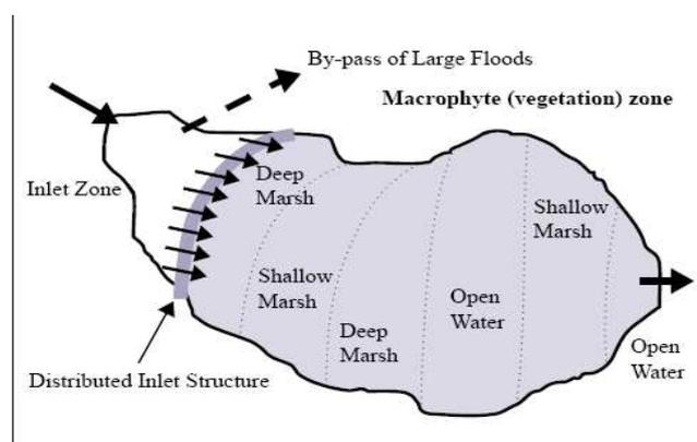
Figure 3: Zones in constructed wetland (WSUD, 2009)
