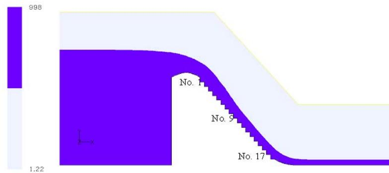
**Figure 4: Free water surfaces obtained by simulation**
