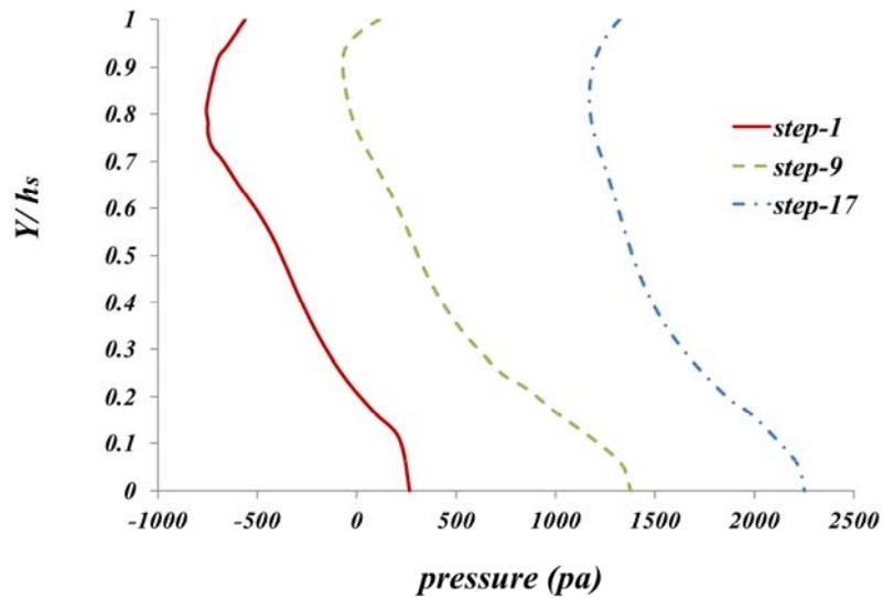
**Figure 7: Pressure profiles on vertical surface**
