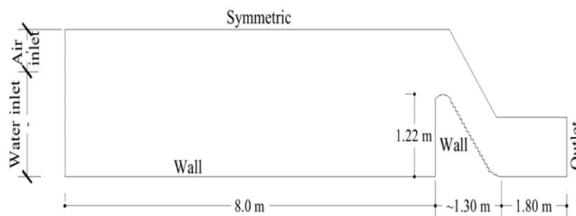
**Figure 3: Boundary condition and dimension of model**
