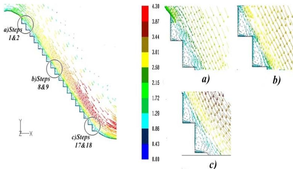
**Figure 5: Velocity vectors (m/s) on (a) After the crest, steps 1&2; (b) At middle of spillway, steps 8&9; (c) Before the toe steps 17&18**
