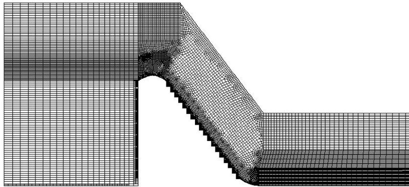
**Figure 2. Mesh domain for step- spillway**
