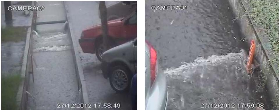
**Figure 4** Tipping flush gate in operation: the flush wave created moment after the gate open (left); the flush wave reaching the end of the monitoring stretch 40 m from the gate about 20 second after the gate open (right).
