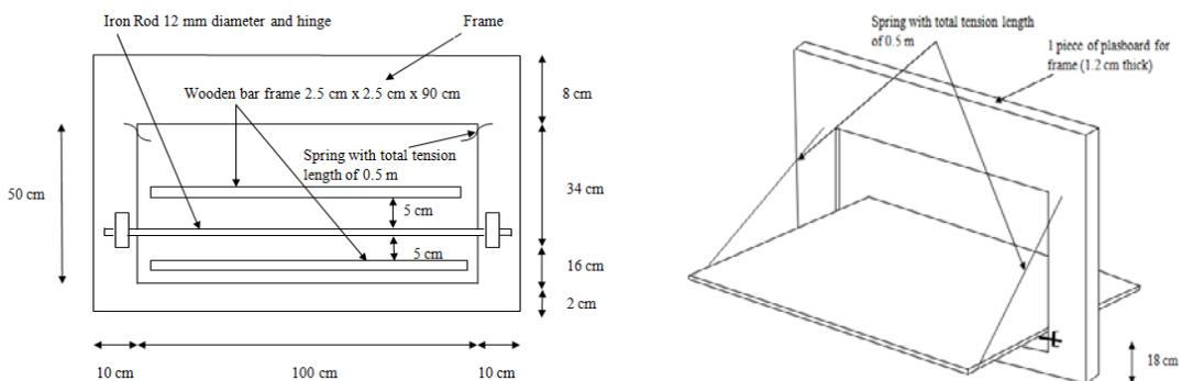
**Figure 3** Front view (left) and isometric view (right) of tipping flush gate used in this study.
