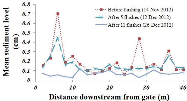
**Figure 5** Changes of mean sediment profile with number of flushes for the period 14 November 2012 to 26 December 2012.
