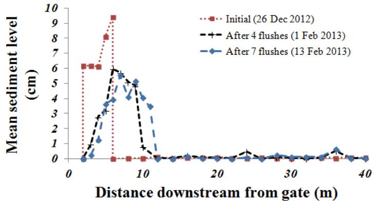
**Figure 6** Changes of mean sediment profile with number of flushes for the period 26 December 2012 to 13 February 2013 after sand was added into the drain.
