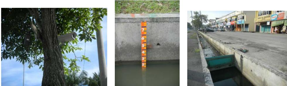
**Figure 2** Site installation: CCTVs (left); stick gage (middle) and tipping flushing gate (right).
