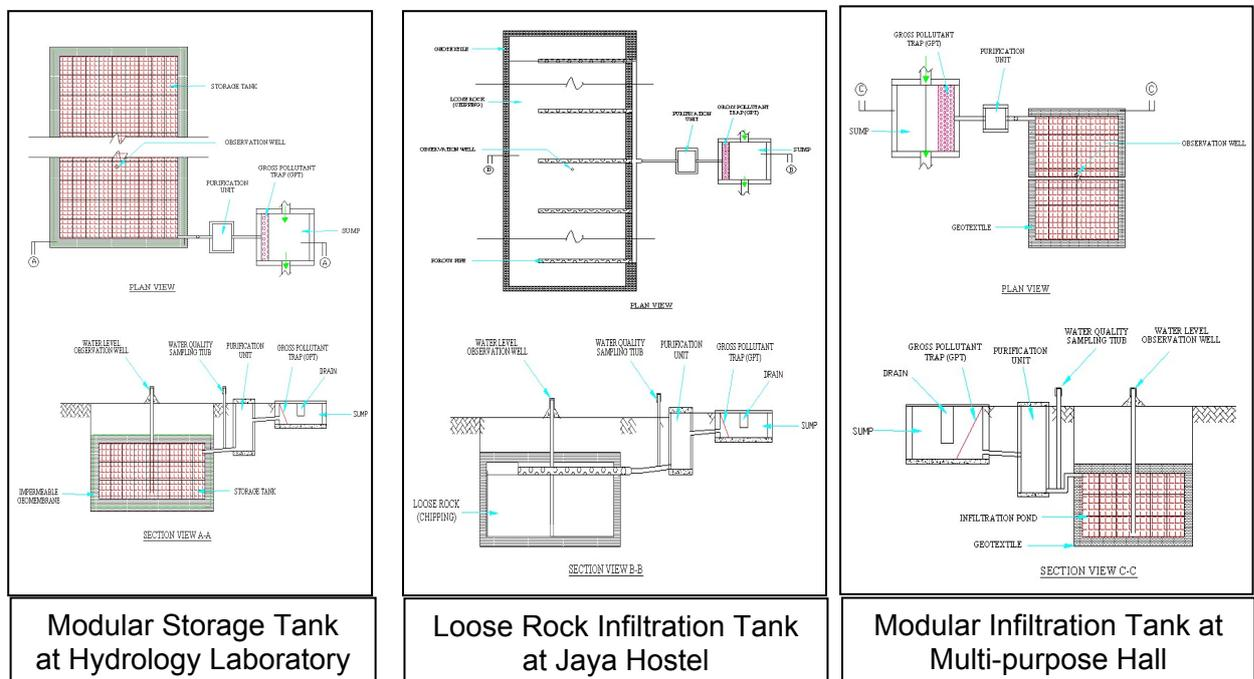
Figure 1 Subsurface on-site detention/retention systems
