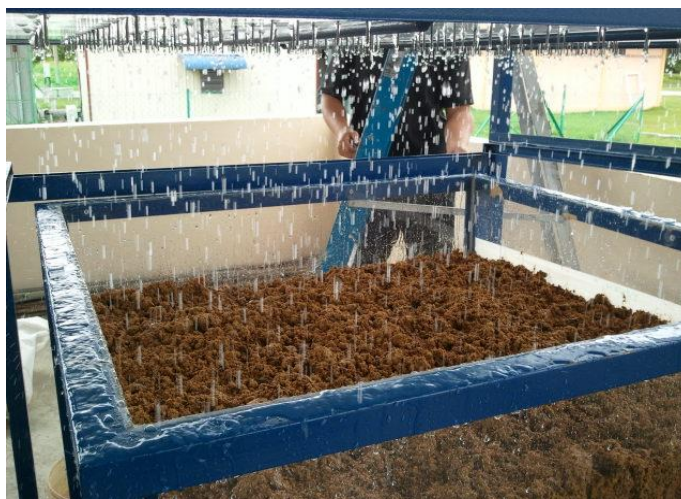
Figure 2 Simulated rainfall on control test bed.
