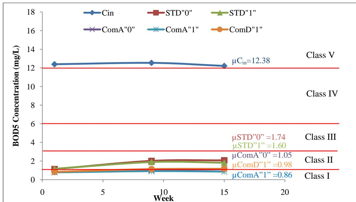
**Fig 1. BOD5 concentration (mg/L) with time for influent (C<sub>in</sub>), standard columns (STD), layer mixed (ComA) and uniformly mixed (ComD)**
