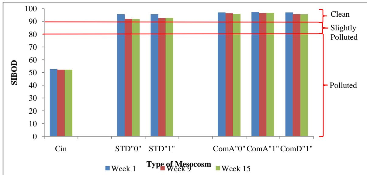
**Fig 3. Comparison of SIBOD performance for STD, Com A and Com D**
