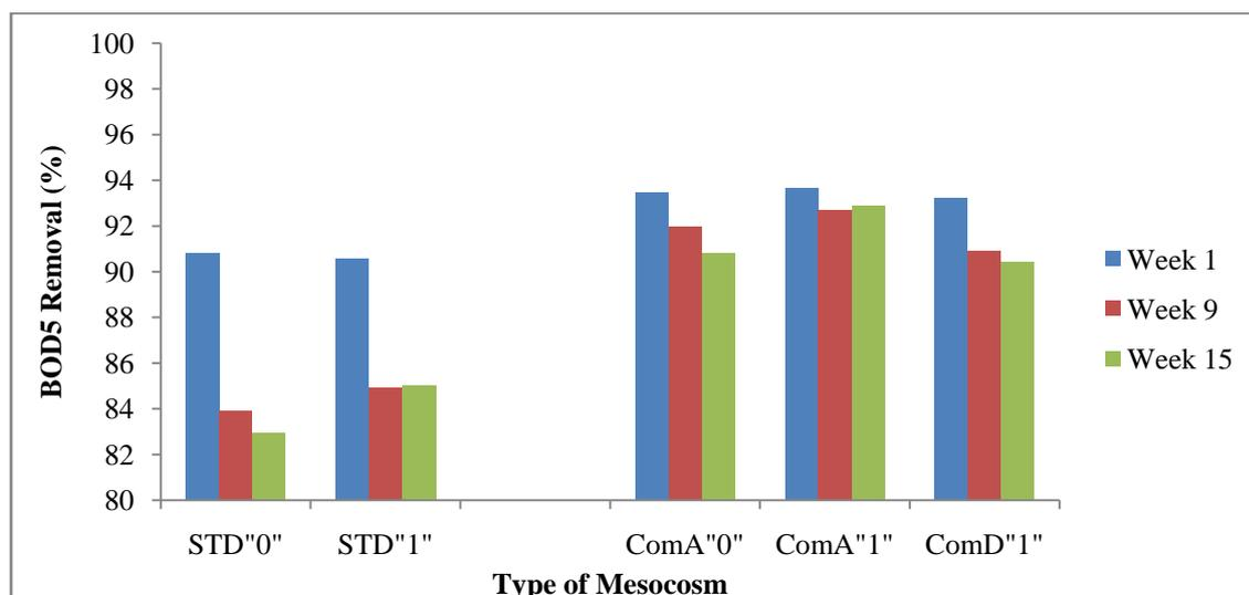
**Fig 2. Comparison of BOD removal (%) from natural runoff by STD, Com A and Com D over time**
