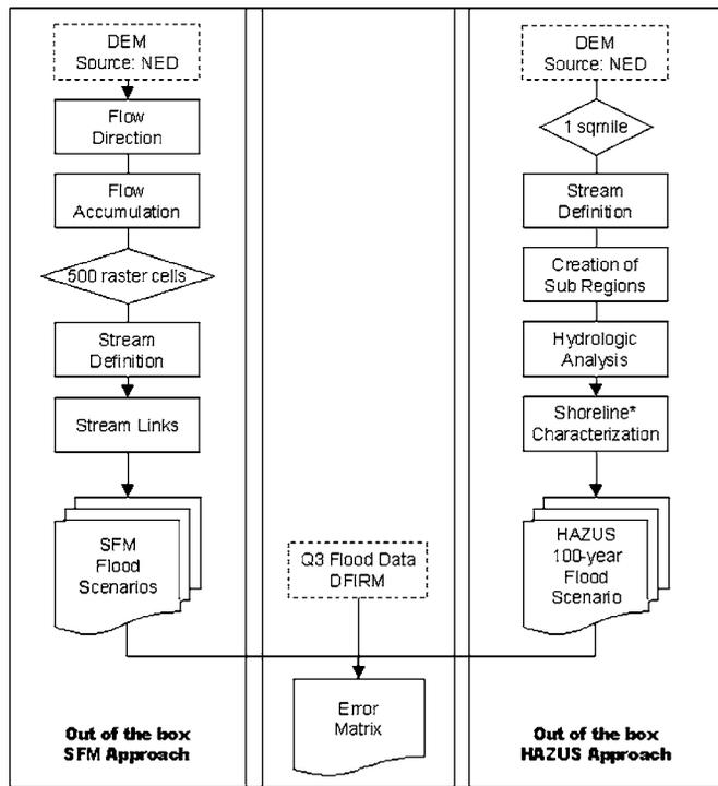
**Fig. 3.** Flow chart of the floodplain modeling and assessment process
