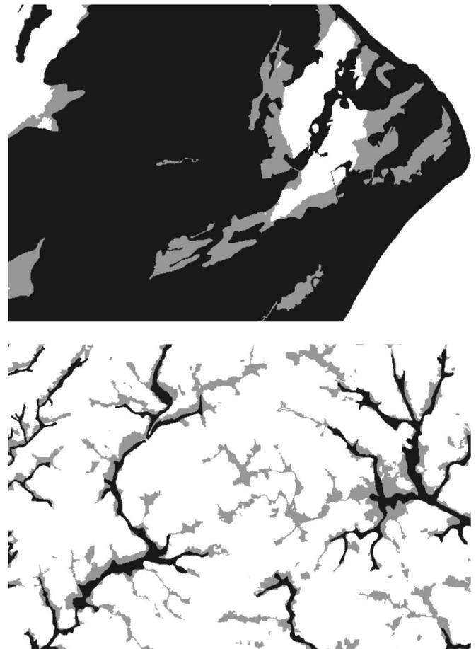
**Fig. 5.** (a) and (b) overprediction of floodplain delineation from modeled output using 30 m DEMs. Fig. 5(a) shows parts of Beaufort County, where HAZUS-MH (gray) overestimates the Q3 floodplain (black). Fig. 5(b) represents an area in Lexington County, where SFM 3.3 (gray) overpredicts the Q3 floodplain (black).
