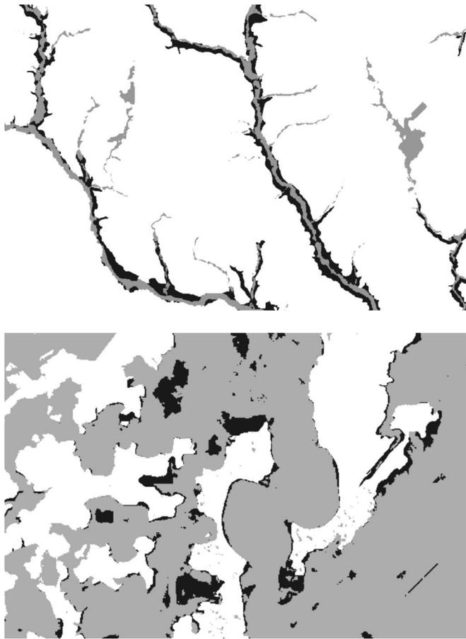
**Fig. 4.** (a) and (b) underprediction of 100-year floodplains using 30 m DEMs. Fig. 4(a) shows parts of Lexington County, where HAZUS-MH (gray) underestimates the Q3 floodplain (black). Fig. 4(b) represents an area in Beaufort County, where SFM 3.3 (gray) underpredicts the Q3 floodplain (black).
