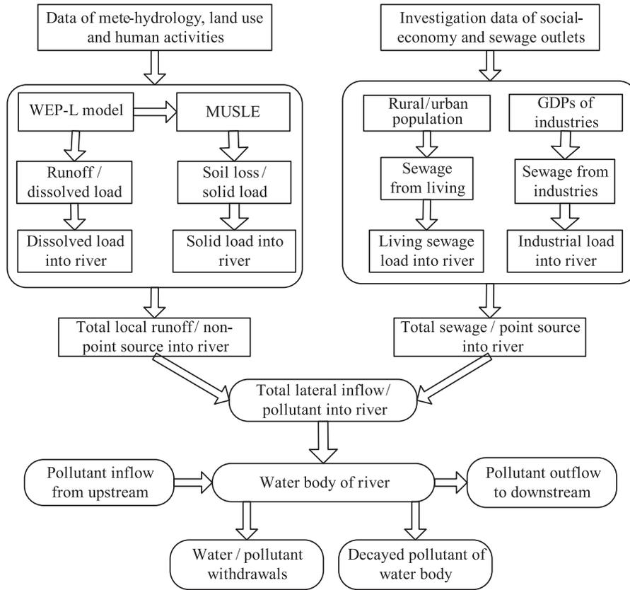
Fig. 2. Computation procedure of water quality module of WEPL.
