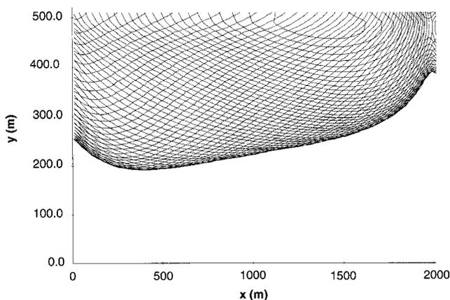
Fig. 2. Flooded area envelope computed by FIVFLOOD
