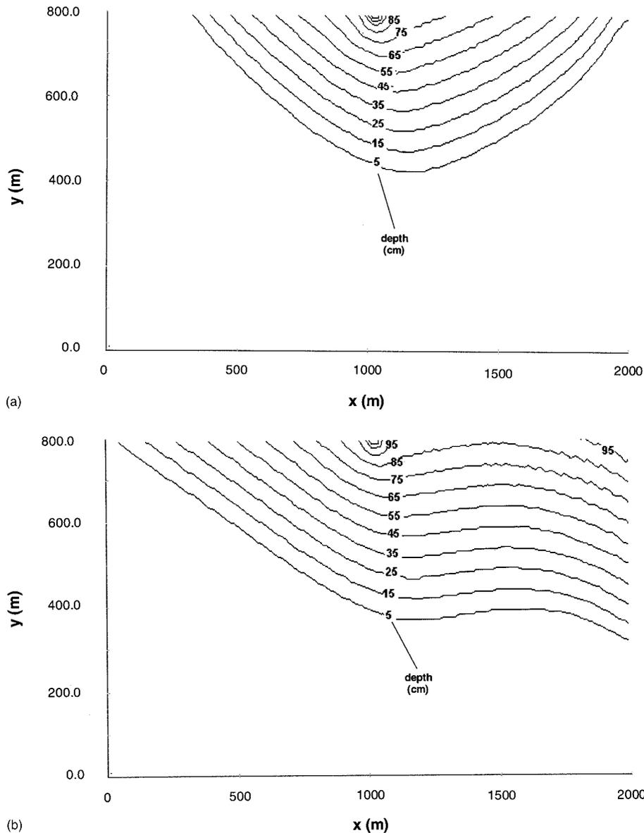
**Fig. 12.** (a) Iso-depth contours for the levee failure test—MCEP— $t = 1,000$  s; (b) Iso-depth contours for the levee failure test—MCEP— $t = 2,000$  s
