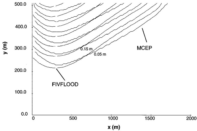
Fig. 3. Iso-depth contours at  $t=3,000$  s (FIVFLOOD versus MCEP)
