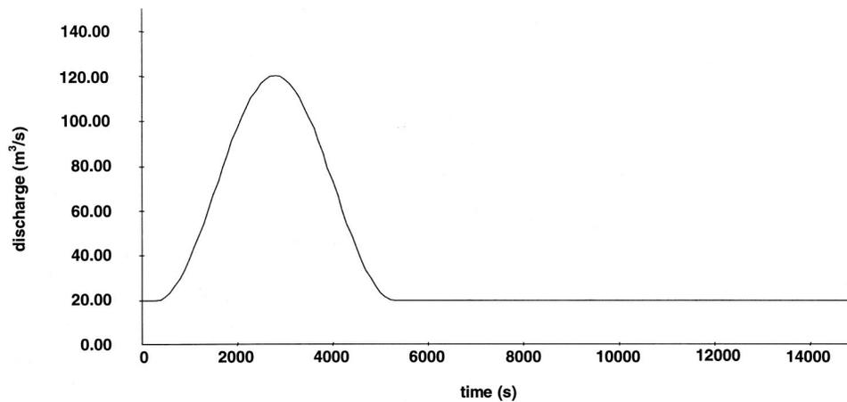
Fig. 1. Inlet hydrograph
