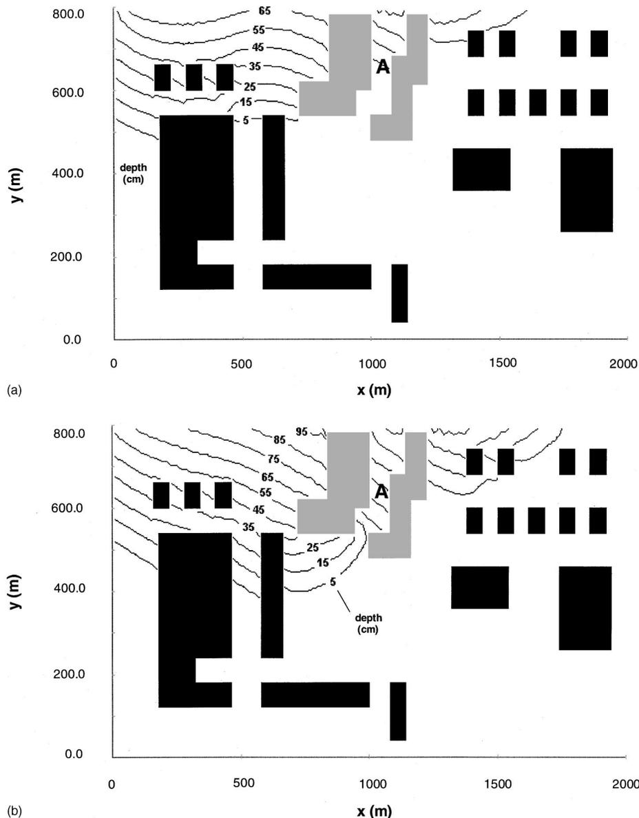
**Fig. 8.** (a) Iso-depth contours—FIVFLOOD (urban area test)— $t=3,000$  s; (b) Iso-depth contours—FIVFLOOD (urban area test)— $t=4,000$  s
