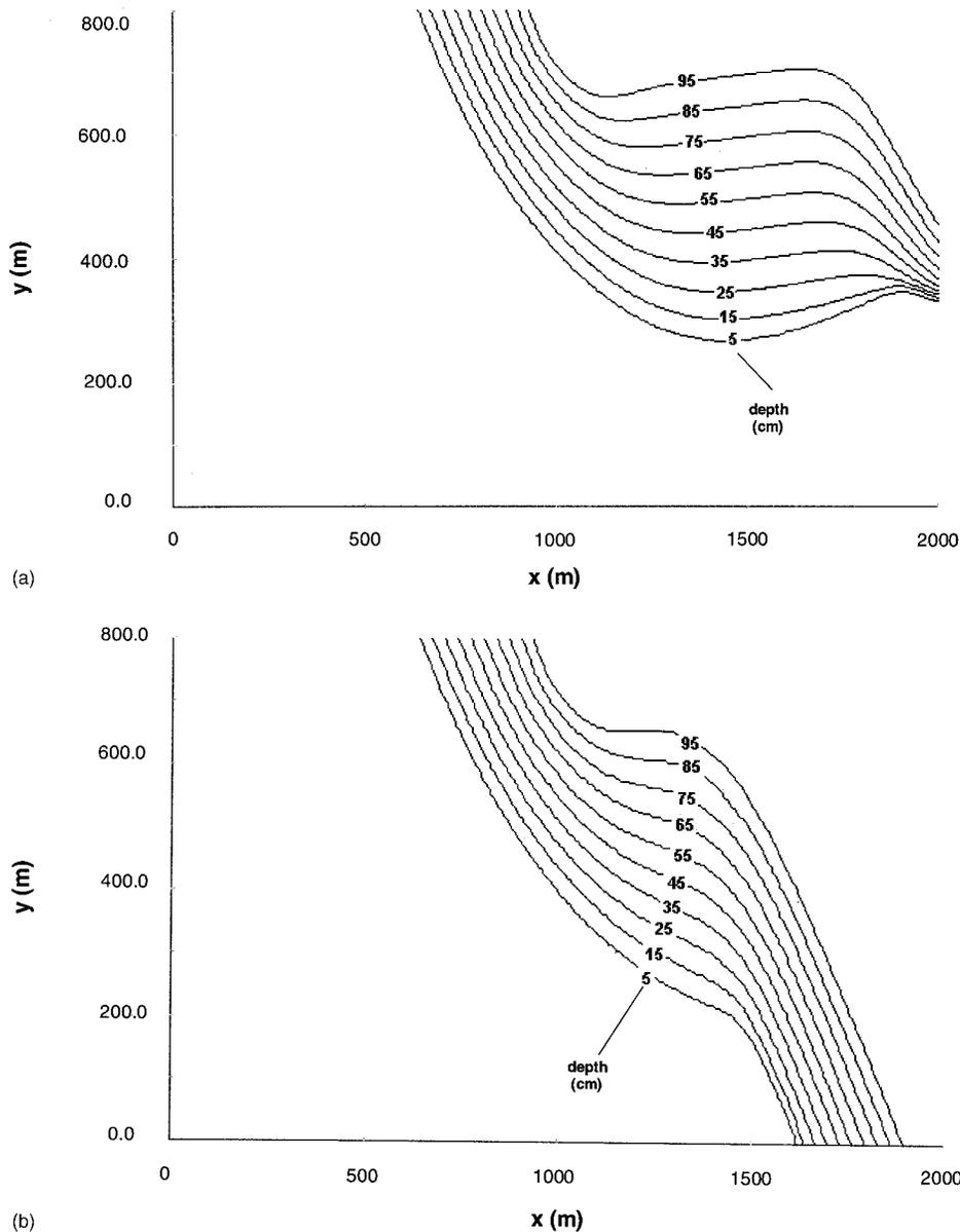
**Fig. 10.** (a) Iso-depth contours for the levee failure test—PA-31— $t = 1,000$  s; (b) Iso-depth contours for the levee failure test—PA-31— $t = 2,000$  s
