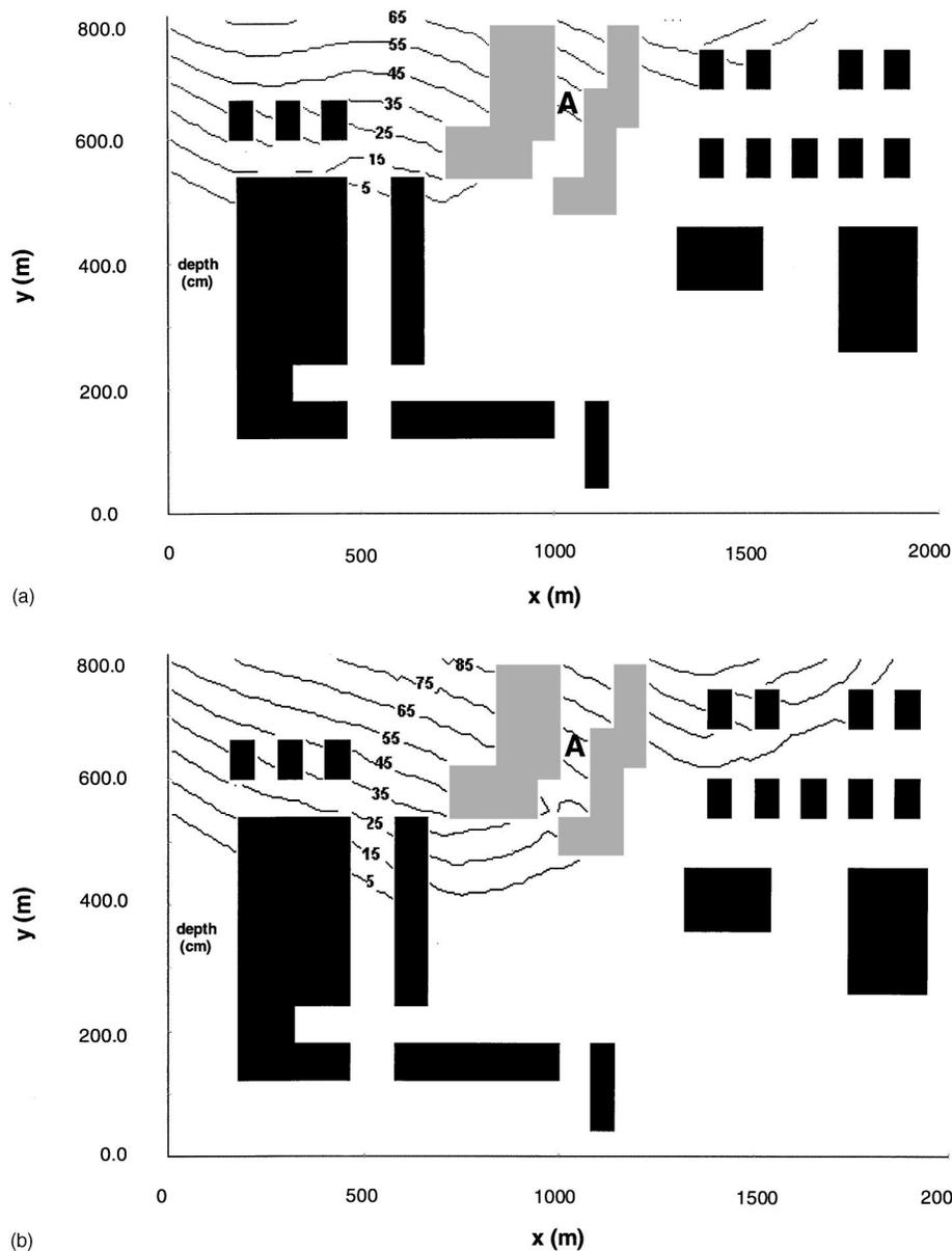
Fig. 9. (a) Iso-depth contours—MCEP (urban area test)— $t=3,000$  s; (b) Iso-depth contours—MCEP (urban area test)— $t=4,000$  s
