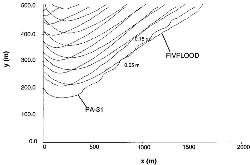
Fig. 4. Iso-depth contours at  $t=3,000$  s (FIVFLOOD versus PA-31)
