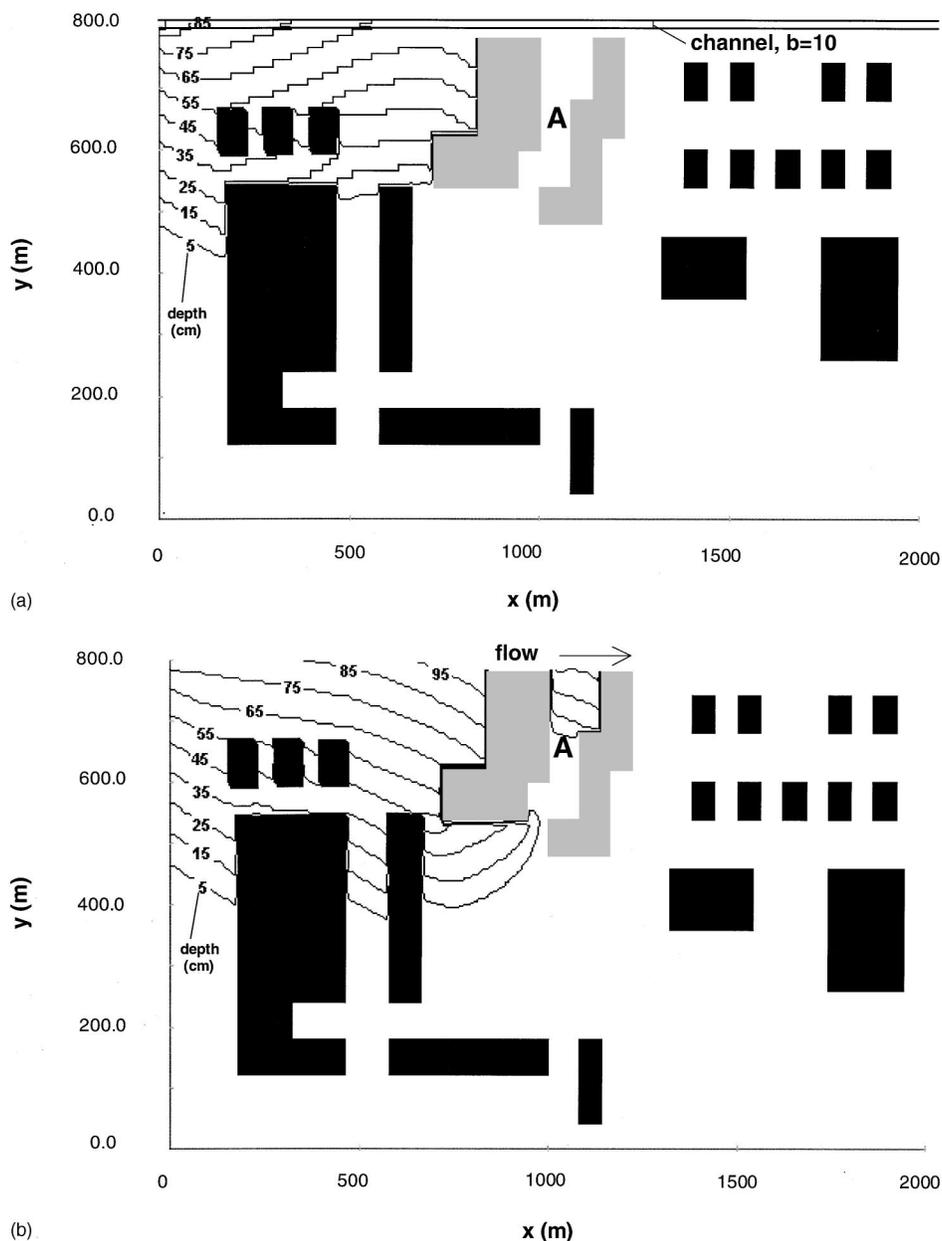
Fig. 7. (a) Iso-depth contours—PA-31 (urban area test)— $t=3,000$  s; (b) Iso-depth contours—PA-31 (urban area test)— $t=4,000$  s
