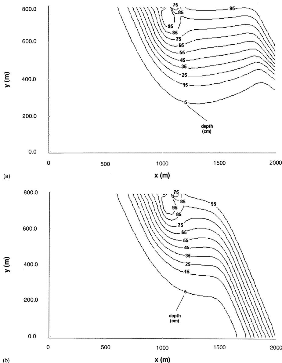
**Fig. 11.** (a) Iso-depth contours for the levee failure test—FIVFLOOD— $t=1,000$  s; (b) Iso-depth contours for the levee failure test—FIVFLOOD— $t=2,000$  s
