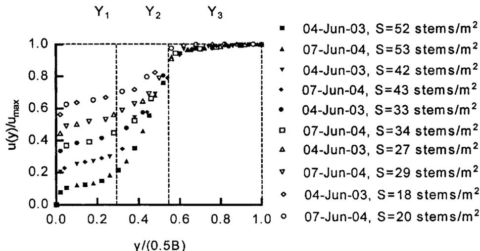
**Fig. 4.** Relative water velocity profile under different reed densities at the measured cross sections
