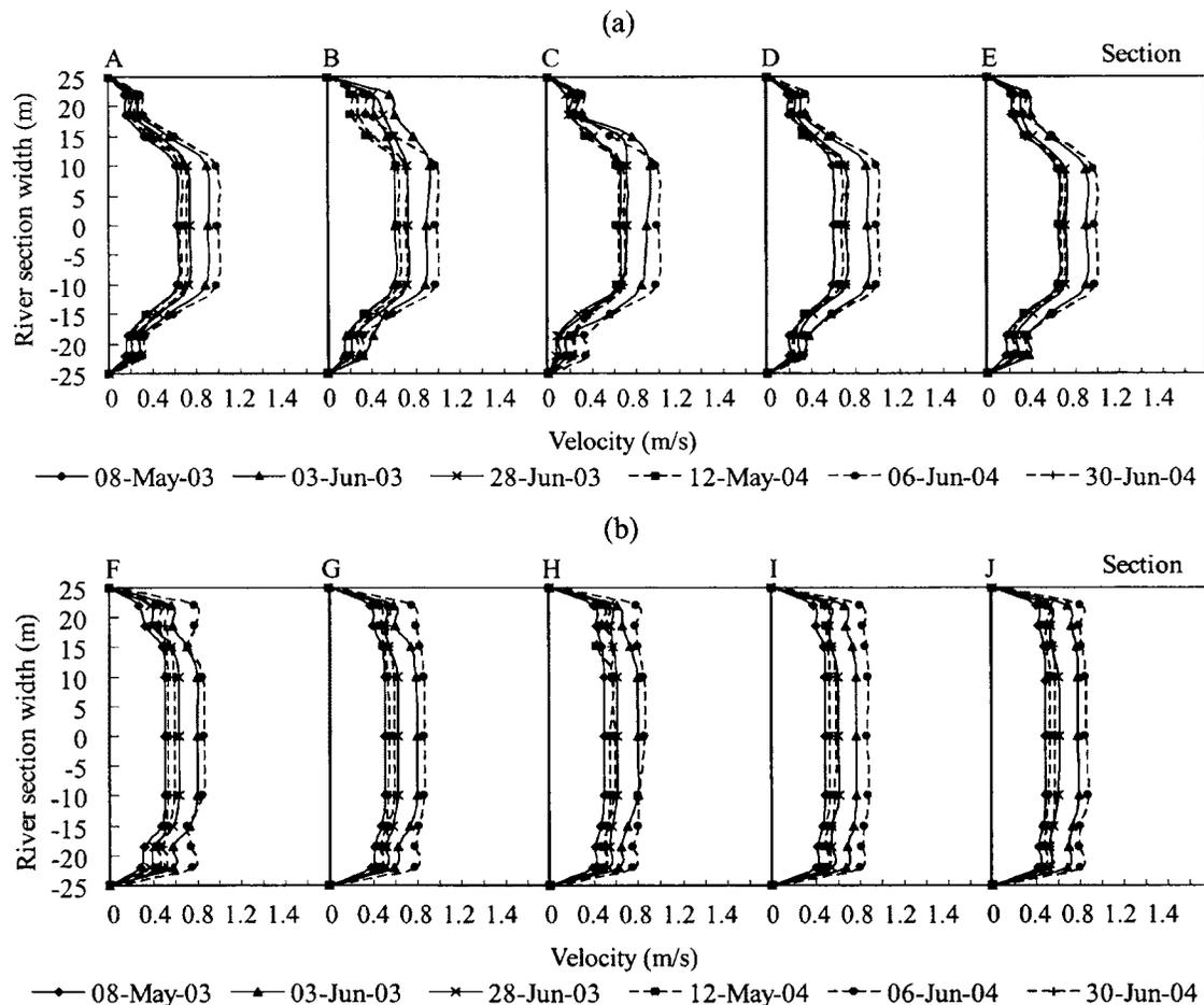
**Fig. 3.** Water velocity profiles during different periods at different cross sections of the Chaodongweigang River reach (a) with or (b) without riparian reed zone
