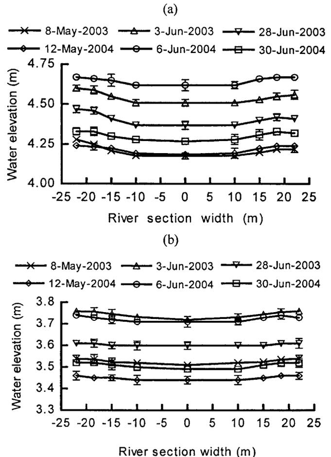
Fig. 6. Distributions of water level at (a) Section B and (b) Section H of the Chaodongweigang River reaches
