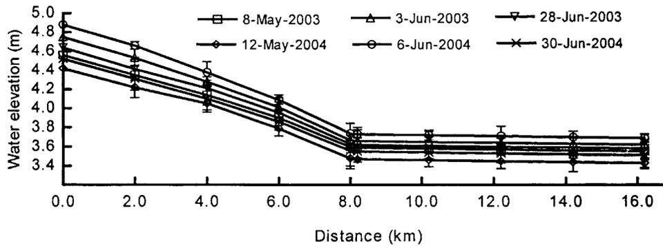
Fig. 5. Water-surface slope during different periods at different cross sections in the center of the Chaodongweigang River reaches
