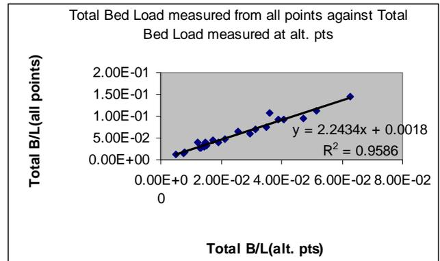
Fig. 3 Total bed load measured at one-meter interval with total bed load measured at two-meter interval.
