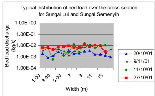
Fig.1 Typical distribution of bed load over the cross section for Sungai Lui and Sungai Semenyih
