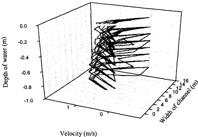
**Figure 3** Transverse velocity profile
