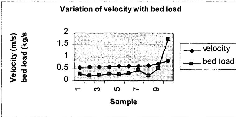
Figure 5 Profile of bed load with velocity
