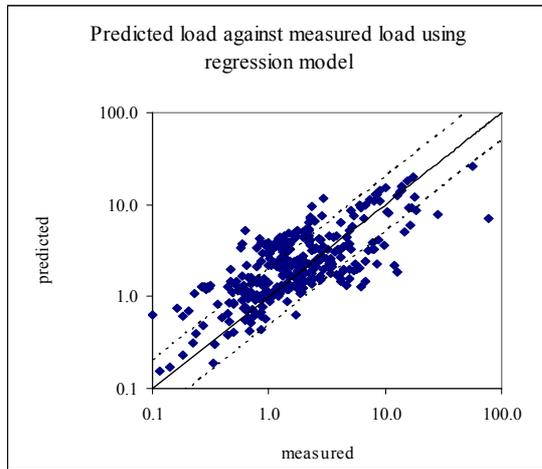
Figure 1 Predicted load against measured load using regression model.
