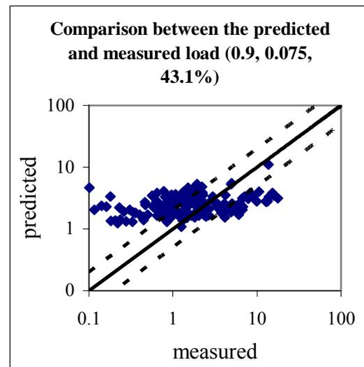
Figure 4 Predicted against measured load (Verified ANN model with alpha = 0.9,  $\eta$  = 0.075 and 8 neurons in the hidden layer) on 181 sets of data).
