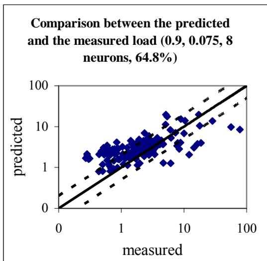
Figure 3 Predicted against measured load (ANN model with alpha = 0.9,  $\eta$  = 0.075 and 8 neurons in the hidden layer).
