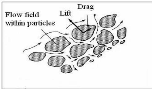
Figure 1 Detachment and entrainment process of particles (Hemphill, 1989).
