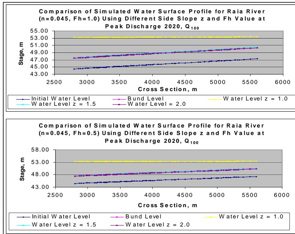
Figure 6 Comparison of Simulated Water Surface Profile of Raia River ( $n=0.045$ ) Using Different Side Slope  $z$  and  $Fh$  Value at Peak Discharge 2020,  $Q_{100}$ .
