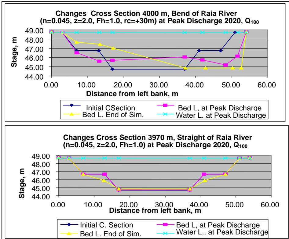
Figure 5 Comparison of Cross Section 4000 m and 3970 m Of Raia River ( $n=0.045$ ,  $Fh=1.0$ ,  $z=2.0$ ) at Peak Discharge 2020,  $Q_{100}$ .
