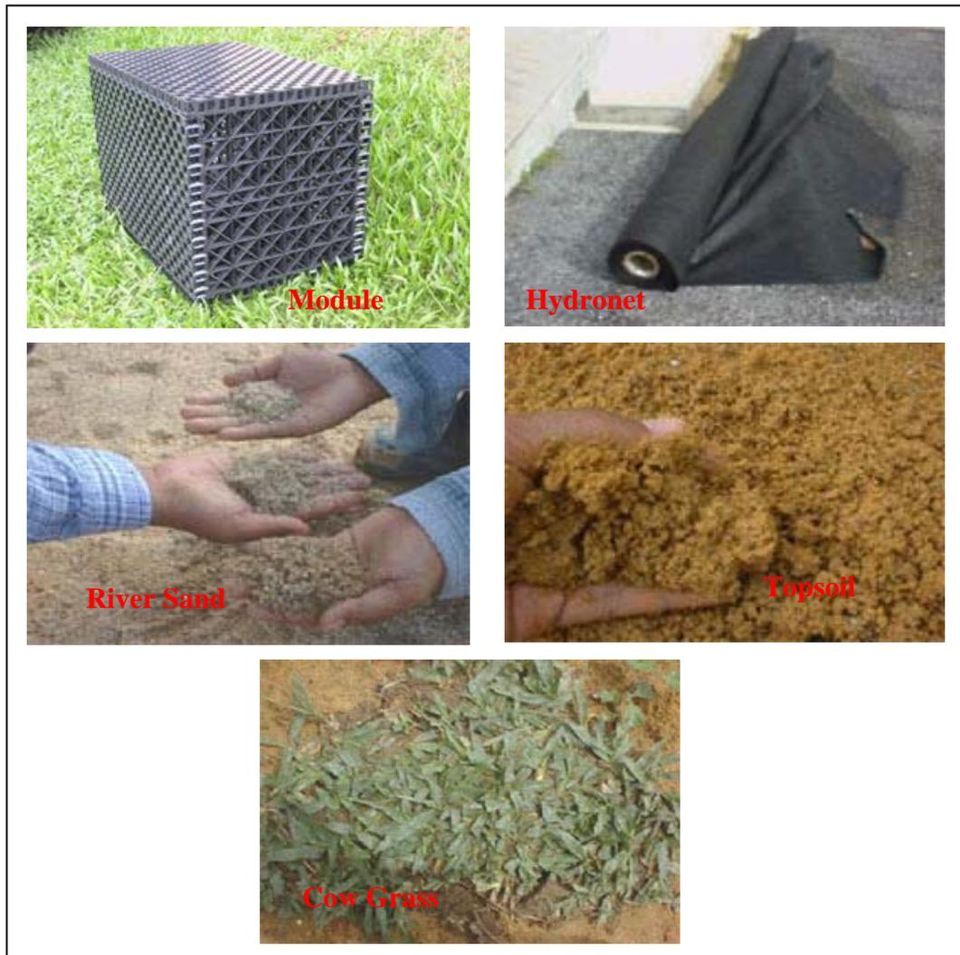
Figure 6 The material of construction of BIOECODS.
