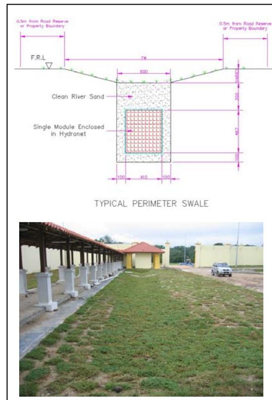
Figure 2 Perimeter Swale.
