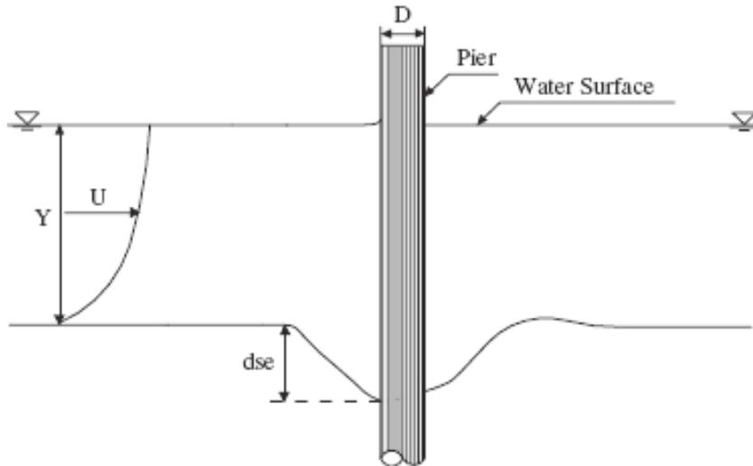
Fig. 1: Flow and local scour around a circular pier (Bateni et al. 2007).
