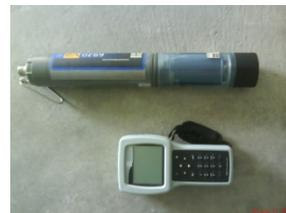
Figure 5 YSI 6920V2 (Top) and YSI 650MDS(Bottom)
