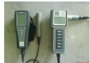
Figure 6 YSI Pro 20 (left) and YSI 60 (right )
