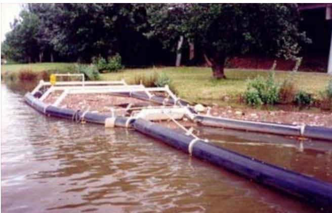
Figure 12 Floating debris trap (Courtesy of stormwater systems, Inc.)
