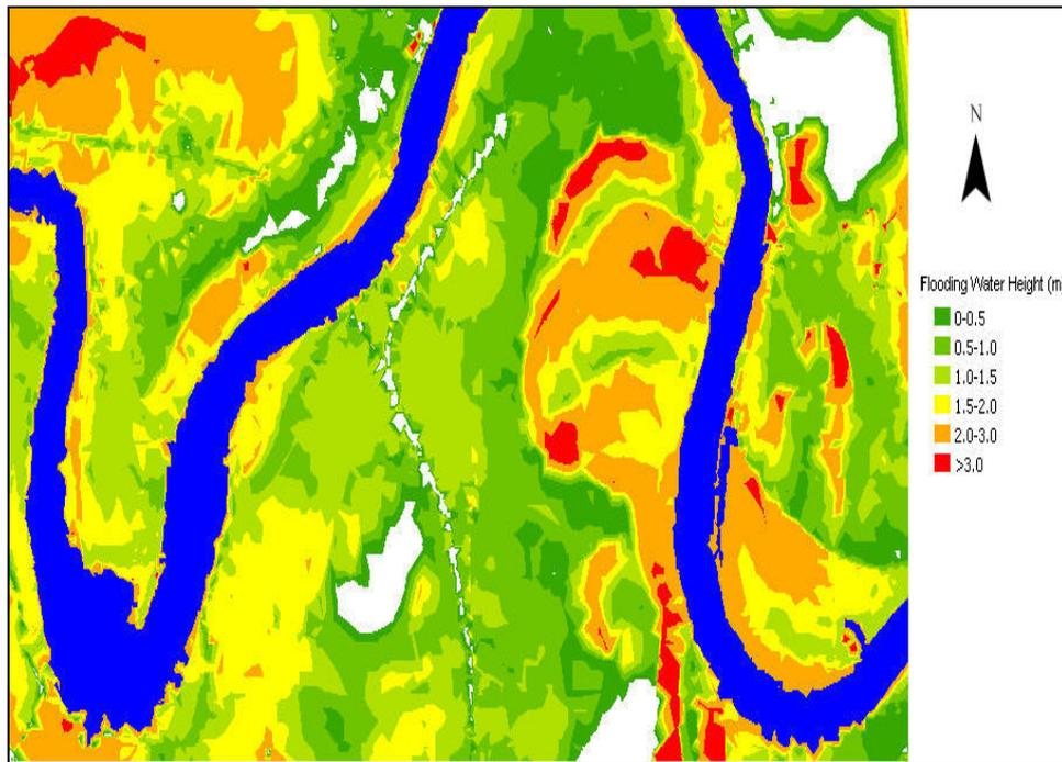
Figure 4 Simulated Inundation Depth Map during 6<sup>th</sup> October 2003 Flood
