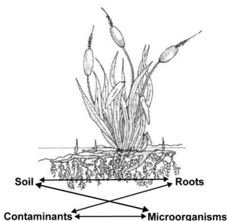
Figure 1 Possible interaction in the root zone of wetlands for wastewater treatment (Stottmeister et al., 2003)
