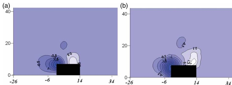
Figure 3 Development of scour hole around abutments in Test A-3 (a) after 5 min and (b) after 30 min.
