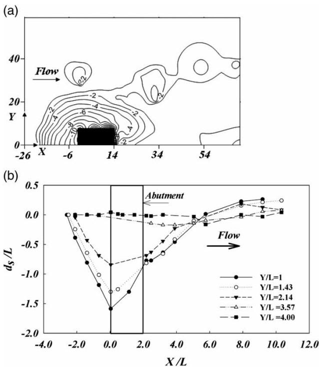
Figure 6 Scour hole around abutment in Test A-3 (a) topography and (b) longitudinal profile.
