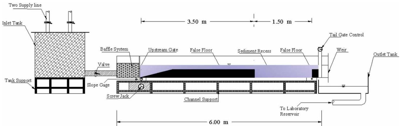
Figure 2 Longitudinal flume section.
