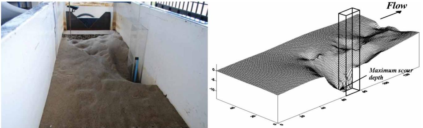
Figure 5 Observed scouring around abutment Test A-3.
