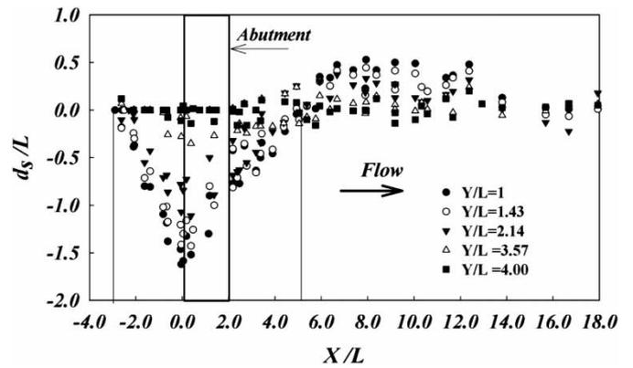
Figure 7 Scour hole around abutments in Test A-1, A-2 and A-3 in different longitudinal sections.
