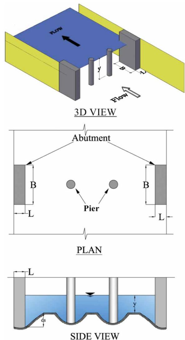
Figure 1 Local scour around abutment and pier.
