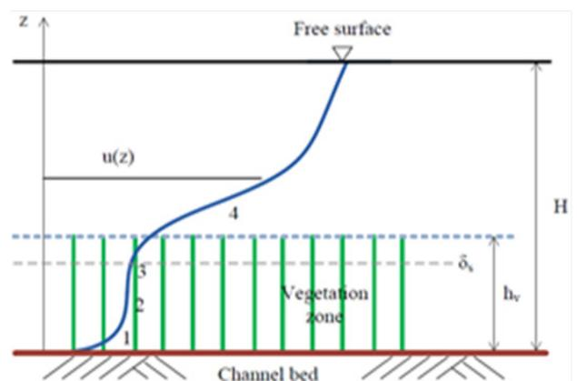
Figure 2. Vertical velocity profile of submerged vegetation.
