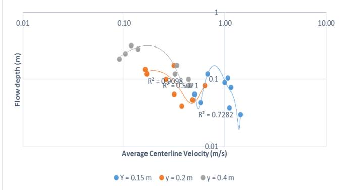
Figure 7: Centerline velocity profiles due to different flow depths.
