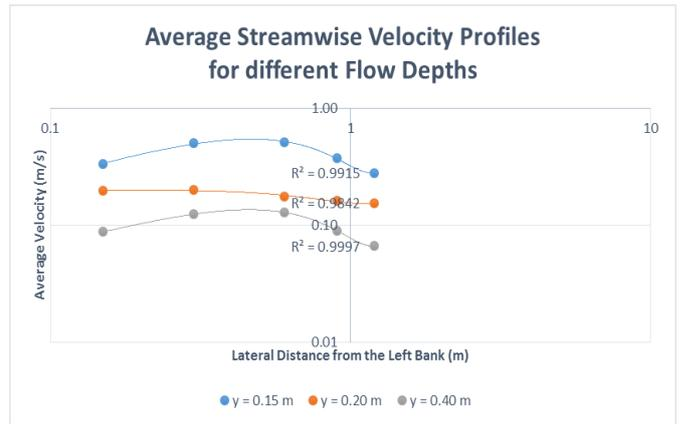
Figure 6. Average stream-wise velocity distribution for the different flow depths.
