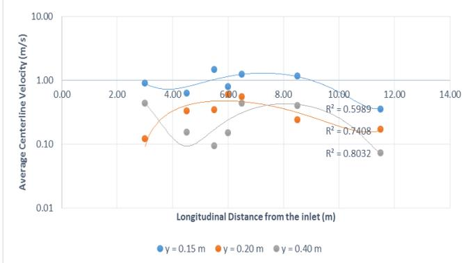
Figure 8: Vertical velocity profile along the channel length reach.
