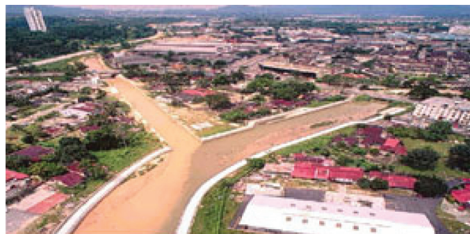
Figure 4 Sedimentation in the river will reduce the hydraulic capacity of river (River Kelang, Kuala Lumpur).
