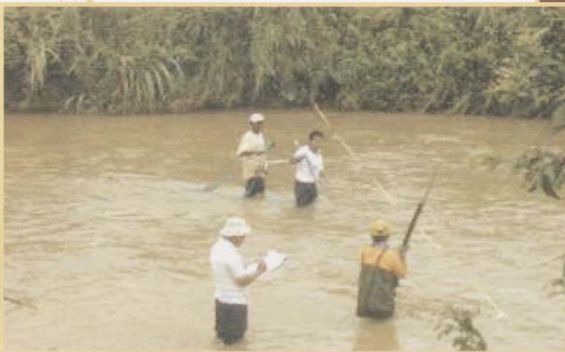
Sediment Load Sampling & Flow Measurement
