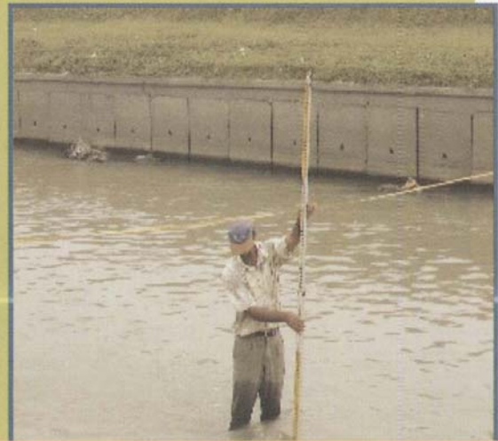
Undergraduate Students During Sediment Transport Measurement at Pari River, Ipoh
