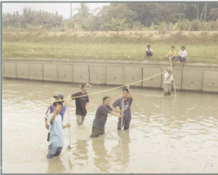
Undergraduate Students During Sediment Transport Measurement at Pari River, Ipoh
