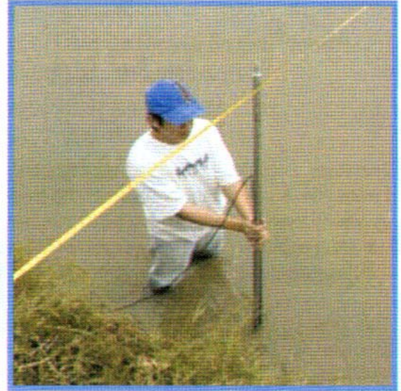
Velocity measurement using electromagnetic current meter
