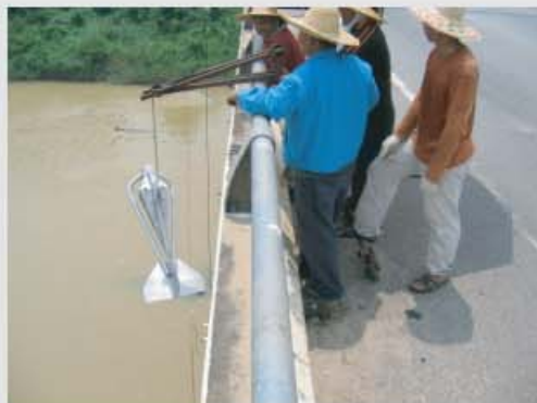
Bed Load Sampling @ Ladang Victoria New Bridge
