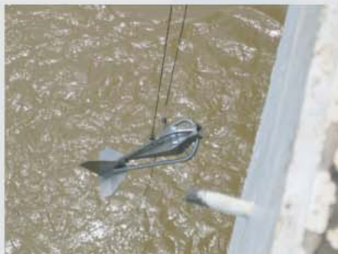
Bed Load Sampling @ Ladang Victoria New Bridge
